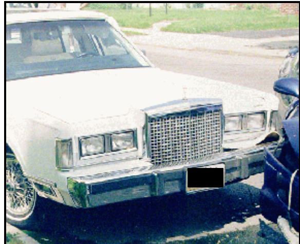
Figure 7: Unoccupied and parked vehicle's front left corner damage from third of three crash sequence events (case photo #14)
