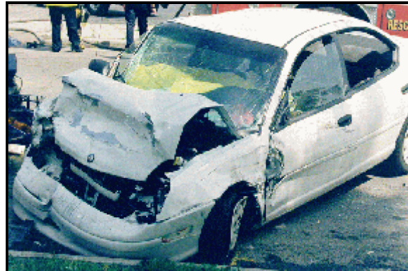
Figure 3: Case vehicle damaged planes, side damage on the left and head-on damage across frontal plane (case photo #03)
