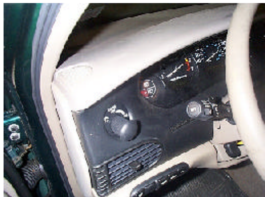
Figure 6 View of the left instrument panel showing the headlight switch which was deformed downward by the driver's left hand
