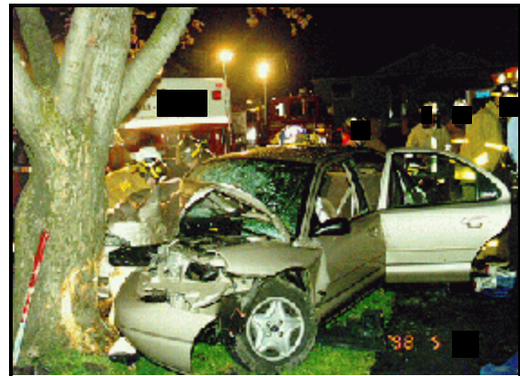
Figure 3: Case vehicle at final rest showing frontal damage from tree impact; Note: tree penetration depth (case photo #05)
