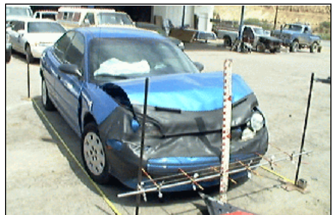
Figure 3. Right front quarter view of frontal damage
