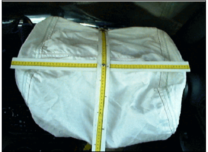
Figure 8. Deployed passenger's frontal air bag
