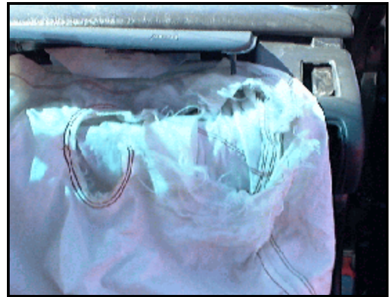
Figure 6. Passenger's frontal air bag damage.
