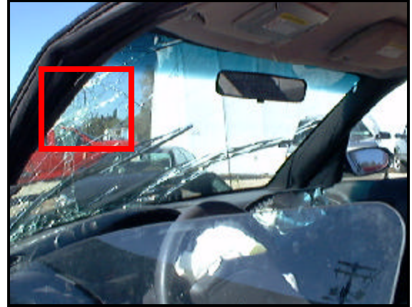
Figure 7. Interior, case vehicle. Box shows location of left arm contact.
