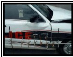
**Figure 4. Sideslap damage to the right side.**
