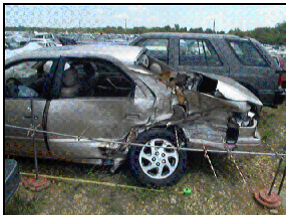
Figure 4: Straight on view of deformation to case vehicle's left side with contour gauge set up; NOTE: integrity loss to back light and door window
