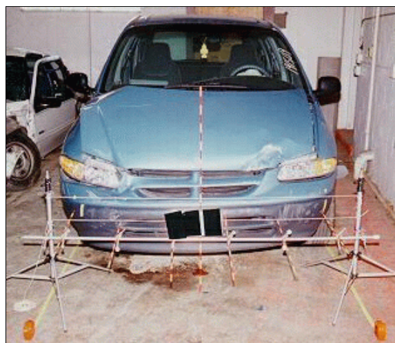
Figure 2: Case vehicle's frontal damage from impact with Intrepid; Note: contour gauge present at bumper level (case photo #12)
