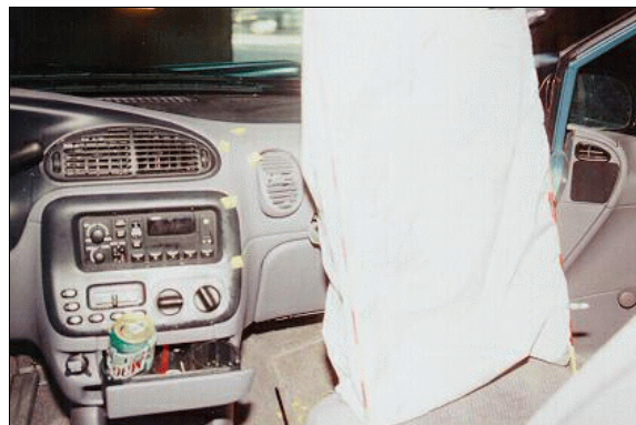
Figure 6: Case vehicle's deployed front passenger air bag showing no obvious occupant contact evidence on air bag's front surface; Note: occupant contacts to center instrument panel (case photo #39)
