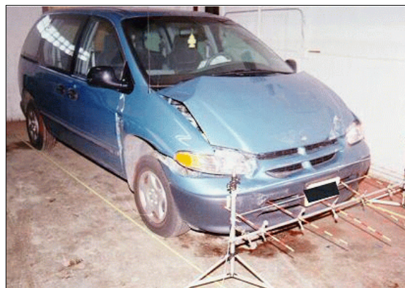
Figure 5: Case vehicle's frontal damage and slight rightward shift viewed from right of front (case photo #25)
