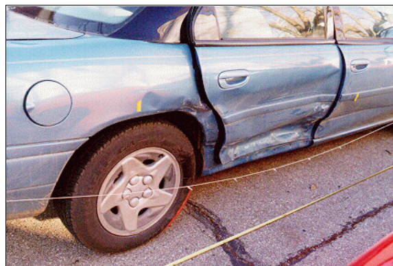
Figure 3: Intrepid's right-side damage; Note: yellow tape indicates width of direct damage (case photo #59)
