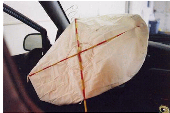
Figure 7: Case vehicle's deployed driver air bag showing only faint marks, smears, and smudges, indicative of only possible occupant contact (case photo #35)
