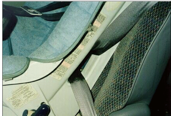
Figure 10: State specialist's photo of case vehicle's convertible child safety seat showing how second seated left passenger in child seat was secured by safety belts (case photo #46)
