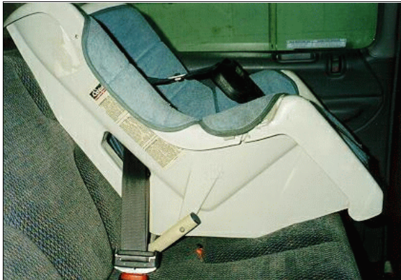
Figure 11: State specialist's photo of case vehicle's convertible child safety seat that was used to restrain second seat left passenger in case vehicle forward facing configuration (case photo #47)
