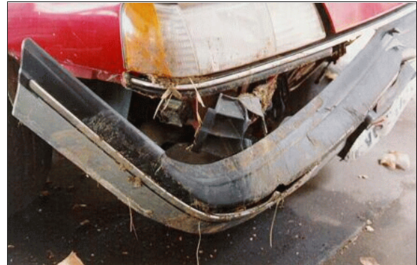
Figure 6: Close-up of damage to case vehicle's front right bumper and undercarriage area from impact with culvert (case photo #14)
