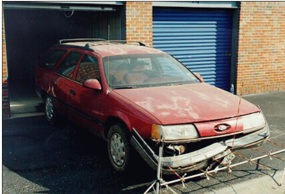
Figure 5: Damage to case vehicle's front bumper and undercarriage from culvert impact viewed from right of front (case photo #13)
