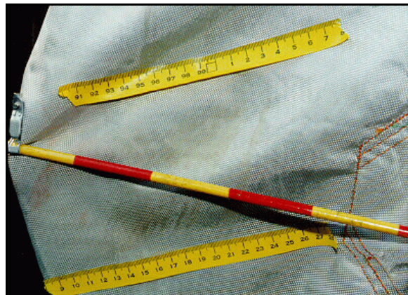
Figure 10: Close-up of case vehicle's driver air bag showing skin transfer on left side (case photo #24)
