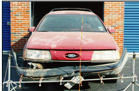
Figure 3: Case vehicle's frontal damage at bumper level and below with contour gauge present; Note: front edge of bumper has been rotated downward and the right side of bumper has been pushed down relative to the left side (case photo #07)
