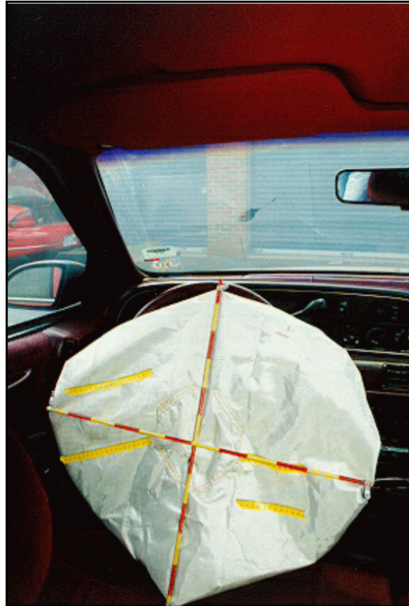
Figure 9: Vertical view of case vehicle's driver seating area showing deployed air bag and greenhouse area; Note: tape indicates skin transfers (case photo #21)
