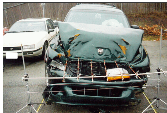
Figure 2: Case vehicle's frontal damage with contour gauge present and positioned to show above bumper crush (case photo #04)
