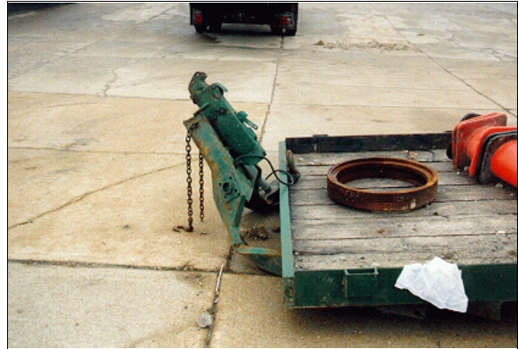
Figure 23: Deformed tongue of flat bed trailer towed by Ford; Note: trailer's tongue was bent upwards when trailer was jammed into back of Ford following trailer's impact by case vehicle's front (case photo #70)
