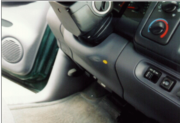
Figure 13: Contact evidence on right side of case vehicle's driver knee bolster (case photo #36)
