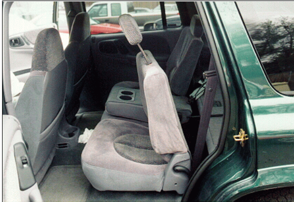
Figure 18: Case vehicle's second seating area showing deformed seat back of second left seat and undeformed seating area where second seat right passenger was seated (case photo #55)
