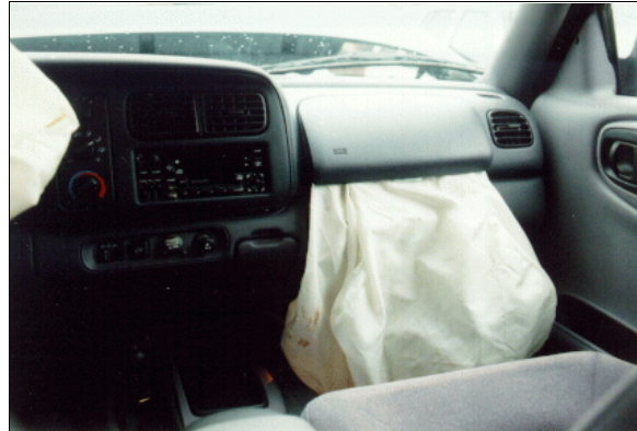
Figure 9: Case vehicle's front right seating area showing front right passenger air bag, which deployed from middle-mounted module, and module's undamaged cover flap (case photo #45)
