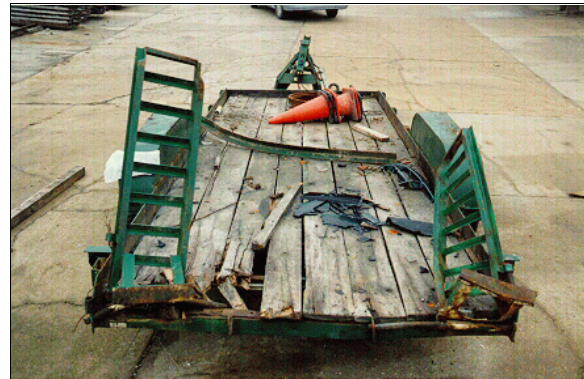
Figure 3: Flatbed trailer towed by Ford showing damaged ramps and wooden floor planks to back of trailer (case photo #72)
