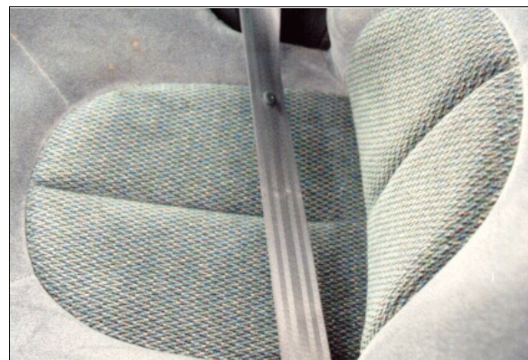
Figure 20: Case vehicle's driver safety belt showing loading evidence on webbing (case photo #39)
