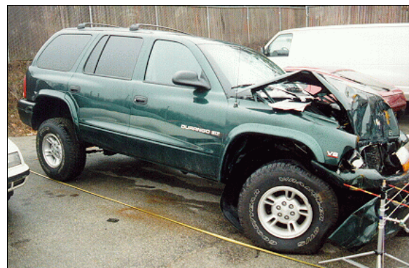
Figure 5: Case vehicle's frontal damage, viewed from right of front, with contour gauge showing bumper level crush (case photo #15)
