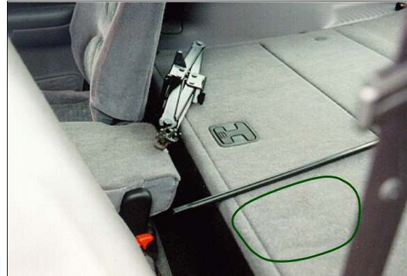
Figure 19: Case vehicle's folded down back seat and base of tire jack that deformed the second seat left's seat back and scraped the folded down area (highlighted) of the back seat (case photo #60)
