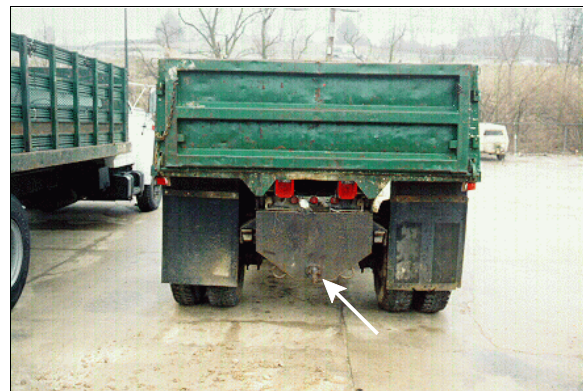
Figure 22: Ford's back showing steel protective plate and repaired hitch assembly (case photo #63)
