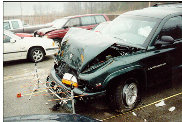
Figure 4: Case vehicle's frontal damage with contour gauge present at bumper level viewed from left of front (case photo #08)
