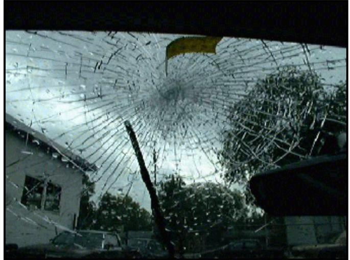
**Figure 7.** Interior, case vehicle. Head contact.
