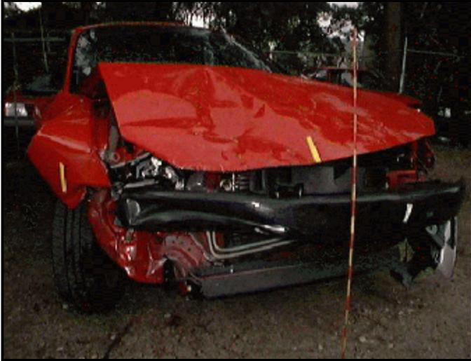
**Figure 4.** Exterior, Vehicle 1, direct damage
