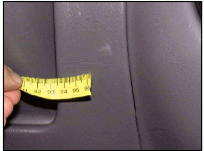
**Figure 9.** Interior, case vehicle. Right knee contact.
