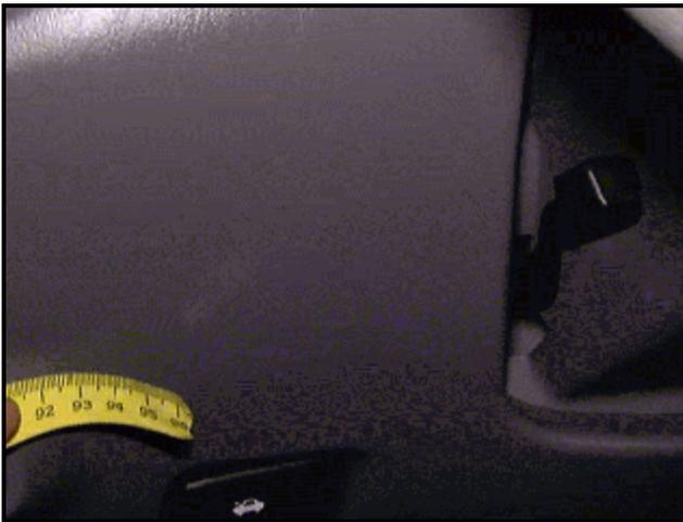
**Figure 8.** Interior, case vehicle. Left knee contact.
