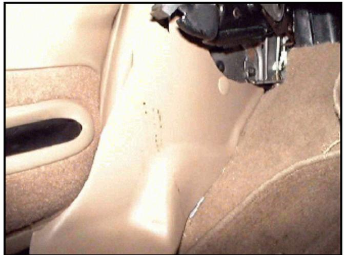
**Figure 8.** Interior, case vehicle. Occupant contact to left side interior surface.
