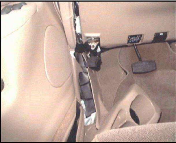
**Figure 7.** Interior, case vehicle. Occupant contact to left instrument panel.
