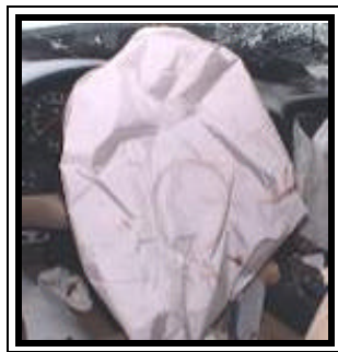
Figure 6. 1999 Chevrolet Corvette redesigned driver air bag.
