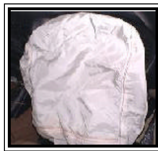
Figure 7. 1999 Chevrolet Corvette redesigned passenger air bag.
