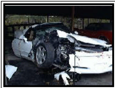
Figure 3. Frontal damage to the 1999 Chevrolet Corvette.
