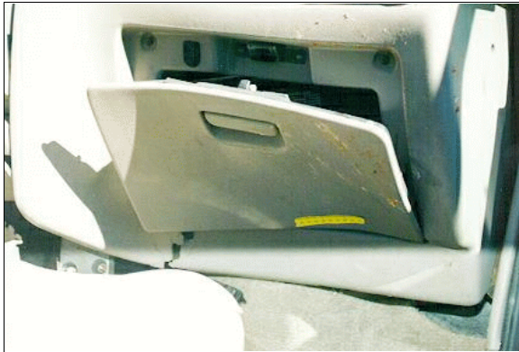
Figure 15: Case vehicle's impacted glove box door and front right knee bolster (case photo #38)
