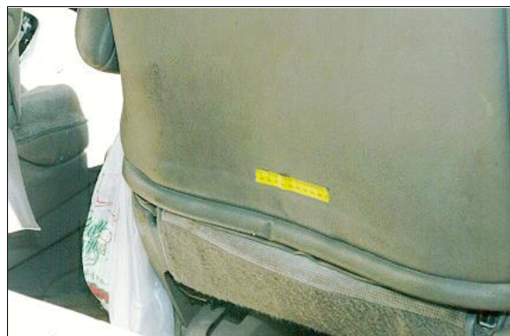
Figure 26: Close-up of lower portion of case vehicle's front right seat back showing evidence of contact by second seat right passenger (case photo #56)
