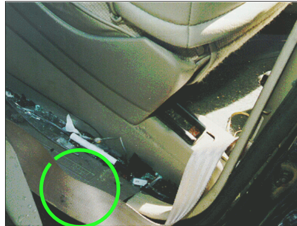
Figure 21: Case vehicle's driver safety belt showing (highlighted) friction scrub (case photo #31)
