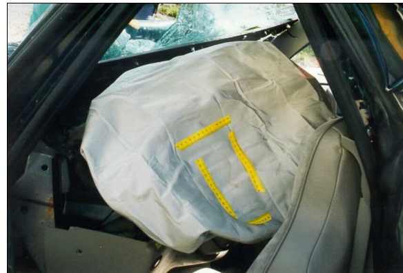
Figure 17: Case vehicle's deployed driver air bag showing (i.e., yellow tape) driver's contact area (case photo #40)
