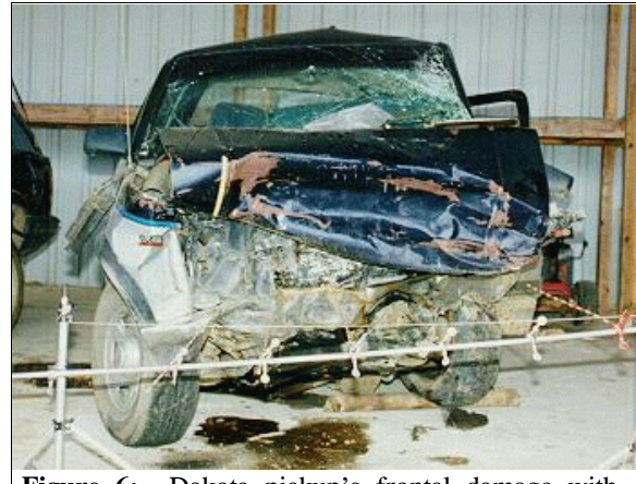
Figure 6: Dakota pickup's frontal damage with contour gauge present (case photo #58)
