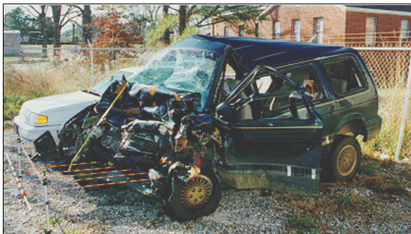
Figure 7: Case vehicle's frontal damaged, viewed from left of front, with contour gauge present (case photo #18)
