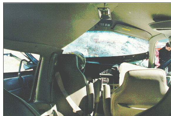
Figure 23: Case vehicle's interior viewed from back showing intrusion into seating area occupied by second seat left passenger (case photo #51)
