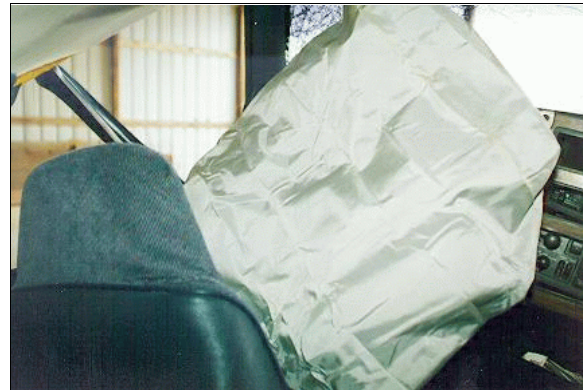
Figure 28: Dakota pickup's deployed driver air bag showing no residual evidence of contact (case photo #76)
