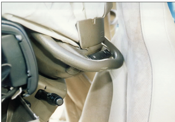
Figure 13: Case vehicle's driver seating area viewed from left showing deployed air bag, air bag module's bottom cover flap, and deformed steering wheel rim against seat back (case photo #42)
