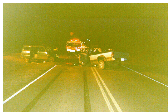
Figure 9: On-scene northward view of the case vehicle and Dakota pickup at final rest positions; Note: Dakota's pre-crash skid marks and post-impact counterclockwise rotation of both vehicles (case photo #13)
