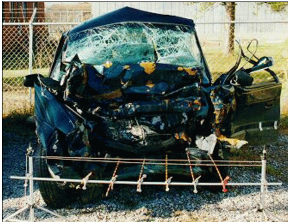
Figure 5: Case vehicle's frontal damage with contour gauge present (case photo #14)
