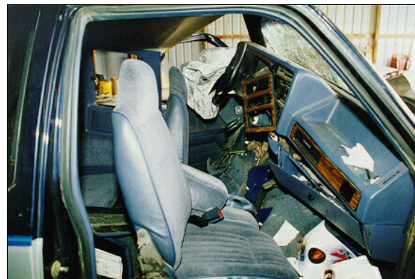
Figure 27: Dakota pickup's front seating area showing massive intrusion into driver's position (case photo #74)
