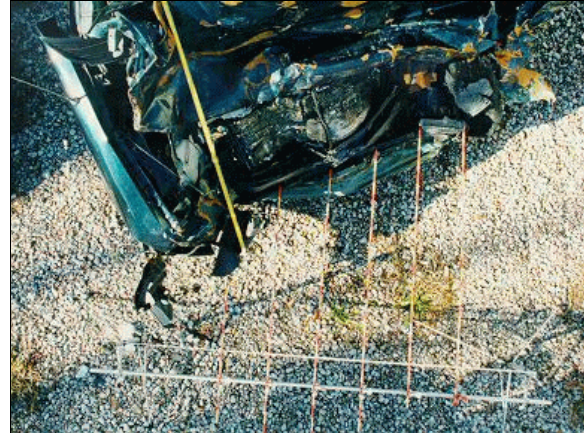
Figure 10: Overhead view of case vehicle’s frontal damage with contour gauge present; Note: offset nature of crush profile (case photo #16)
