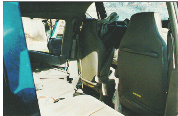
Figure 24: Case vehicle's second row seating area; Note: intrusion to left side and contacts to lower portion of front seat backs (case photo #50)
