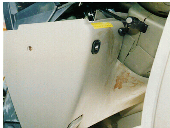
Figure 14: Close-up of case vehicle's driver knee bolster showing contact evidence from driver's knee (case photo #27)
