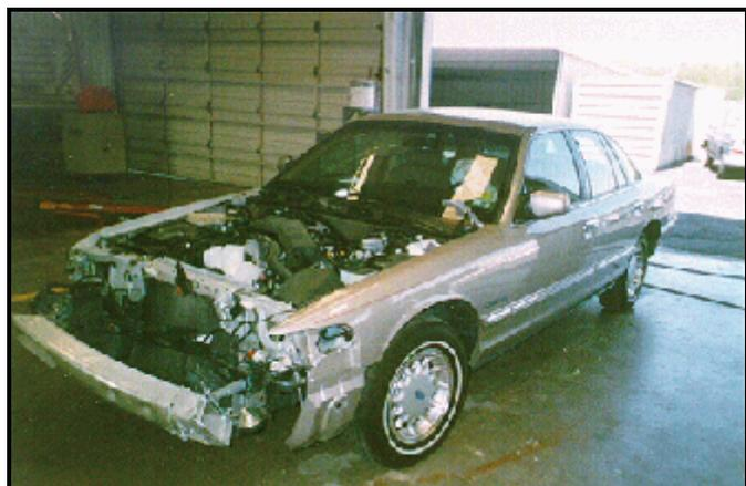
**Figure #1:** Case vehicle's frontal damage viewed from left;
