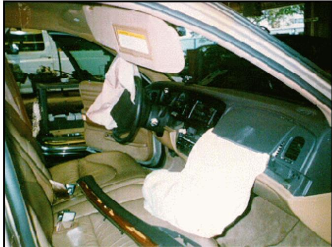
**Figure #5:** Interior of case vehicle's showing deployed air bags; Note: broken piece of dash trim on seat and unknown mark on front right air bag module's cover flap.
