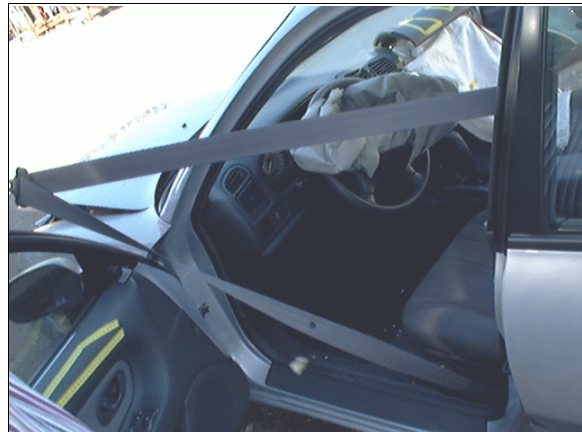
Figure 15: Case vehicle's driver safety belt showing no visible evidence of loading on belt's webbing (case photo #52)
