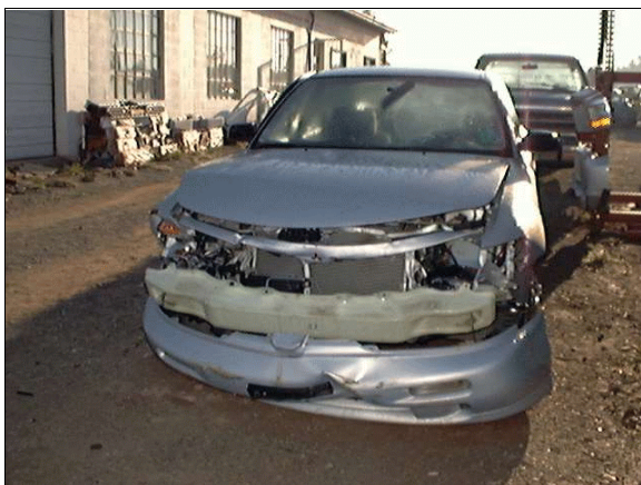
Figure 2: Case vehicle's frontal underride damage from impact with back of Dodge truck (case photo #05)
