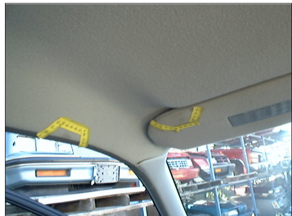
Figure 7: Contact evidence to case vehicle's left roof side rail and driver's sun visor (case photo #26)
