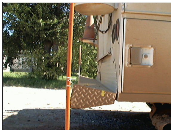
Figure 16: Reference line view from right of Dodge truck showing back bumper's upward rotation (case photo #61)
