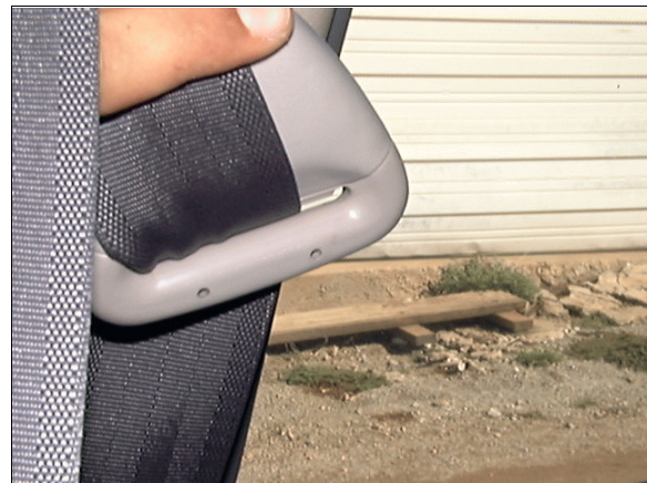
Figure 13: Close-up of "D"-ring for case vehicle's front right safety belt showing no evidence of loading (case photo #29A)
