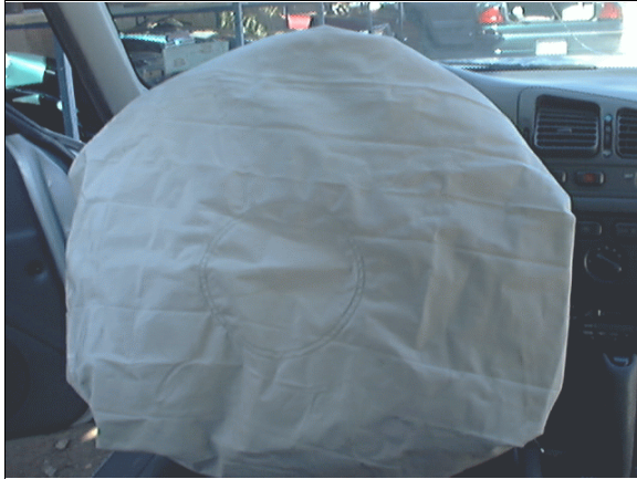
Figure 11: Case vehicle's deployed driver air bag showing no visible evidence of contact on air bag's fabric (case photo #38)
