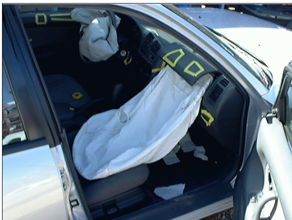
Figure 8: Case vehicle's front seating area showing deployed driver and front right passenger air bags and front right air bag module's cover flap with discounted evidence of contact (case photo #20)
