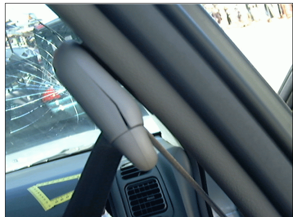
Figure 9: Case vehicle's front right safety belt showing separation to "D"-ring's encasement; Note: cracked windshield glazing in background (case photo #31)
