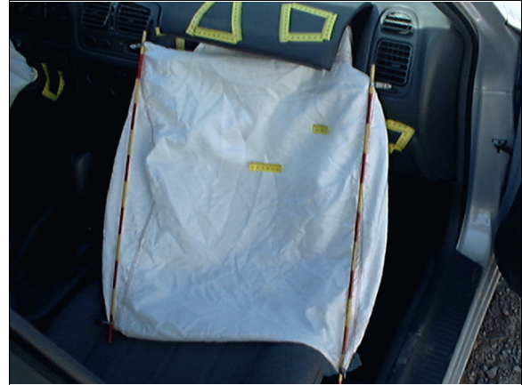
Figure 12: Case vehicle's front right passenger air bag showing areas (i.e., yellow tape) of oil and skin transfers to fabric's upper right quadrant from front right passenger; Note: highlighted possible contact evidence on cover flap was discounted (case photo #44)
