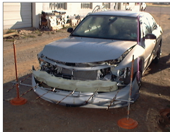
Figure 3: Case vehicle's front underride deformation viewed from left of front with contour gauge present (case photo #09)
