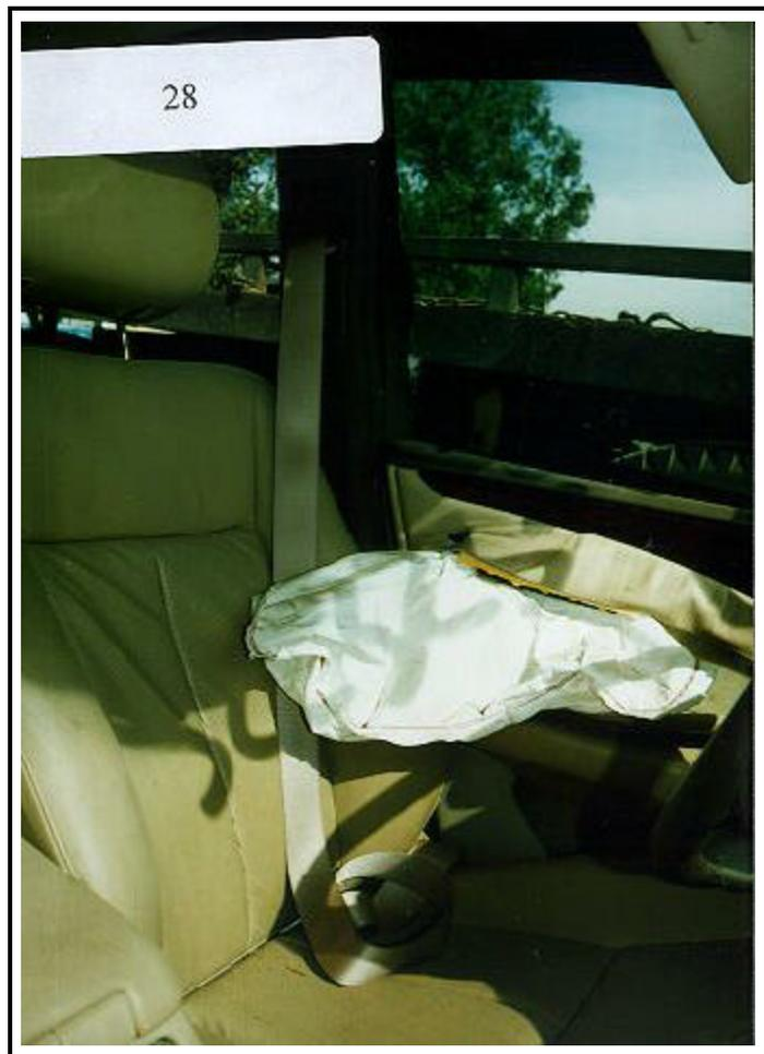
**Figure 2.** Driver's side ETR and air bag.
