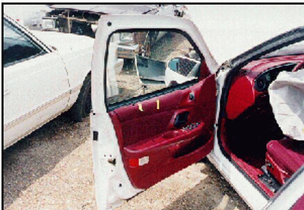
Figure 11: Interior view of case vehicle's left front door; Note: yellow tape defines area of skin transfer and body oil deposits; also note the absence of heavy im-pact to the door panel and door latch (case photo #14)
