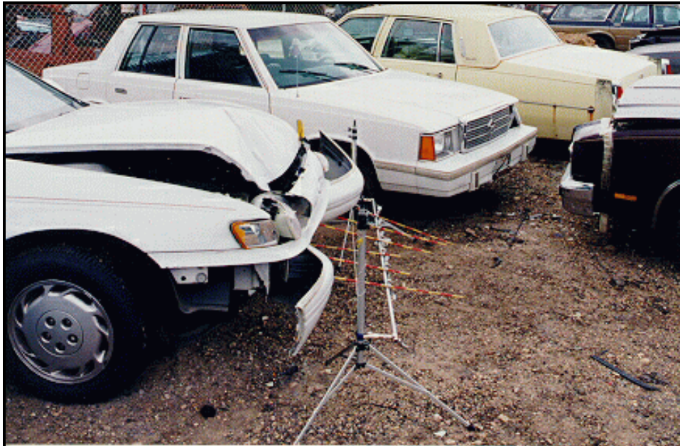
Figure 14: Reference line view of case vehicle's frontal damage from right (case photo #13)
