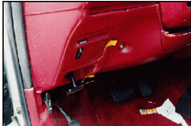
Figure #10: Case vehicle's left lower instrument panel; Note: indications of occupant contact and the down-ward displacement of the parking brake release handle (case photo #18)
