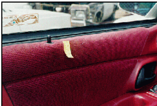
Figure 12: Close-up of case vehicle's left front door panel; Note: yellow tape indicates beginning (on towards the front) of skin transfer and body oil deposits on the window sill; note also the absence of heavy contact to the door panel(case photo #15)
