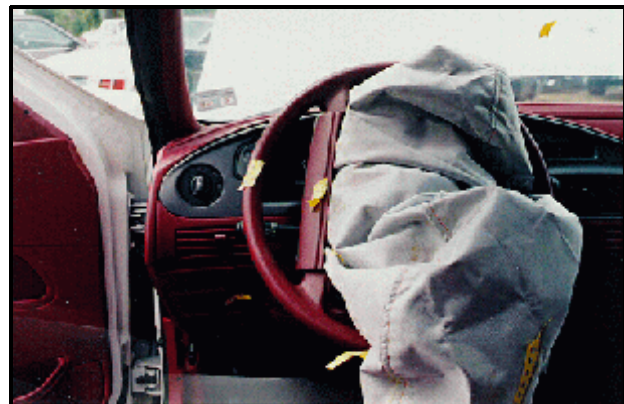
Figure 7: Lower cover flap of case vehicle's driver side air bag module (steering wheel rotated 90 degrees clockwise); Note: yellow tape indicates suspected occupant contact points (case photo #23)
