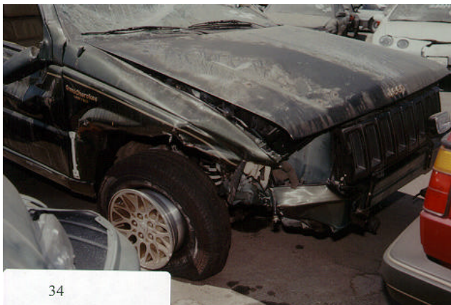
Figure 1. Right front bumper corner damage to V1.
