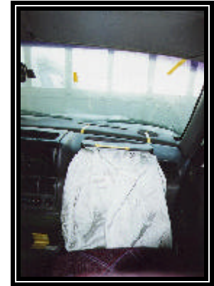
Figure 1. Deployed passenger air bag and resulting damage to the windshield.
