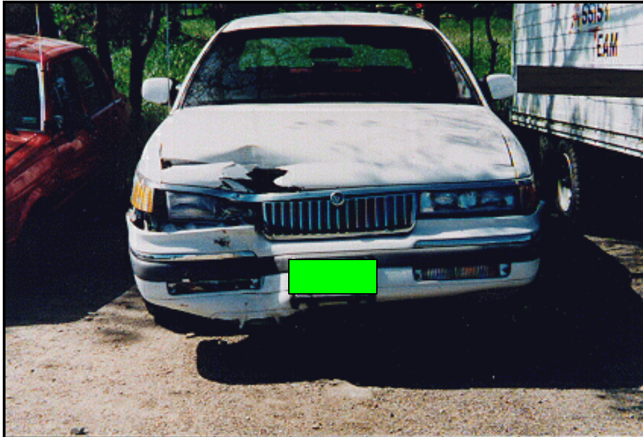
Figure 2#: Case vehicle's frontal damage from impact with wooden utility pole (case photo #02)
