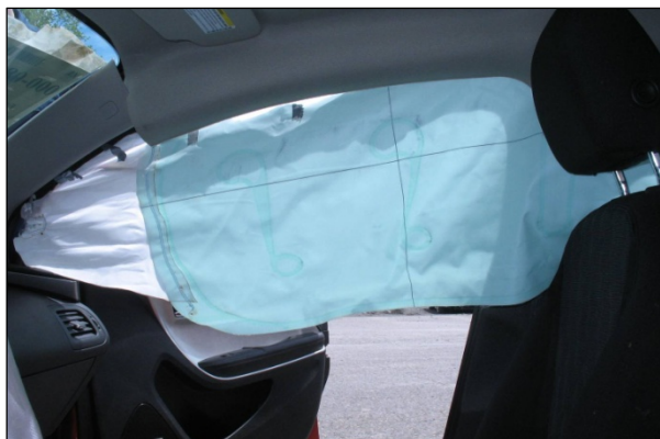
Figure 10: Front row coverage of the deployed right IC air bag.
