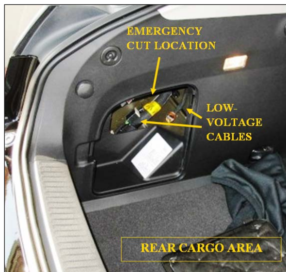
Figure 14: Emergency cut location for 12-V battery. Exemplar vehicle depicted.
