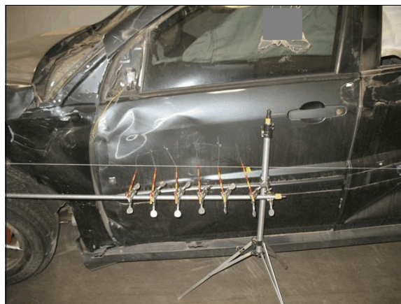
Figure 4: Damage on the left front door of the Chevrolet from the secondary impact by the Ford
