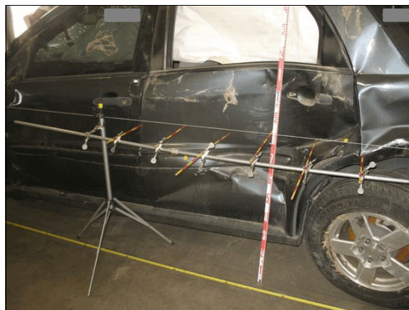
Figure 3: Damage on the left rear door of the Chevrolet from the initial impact by the Ford
