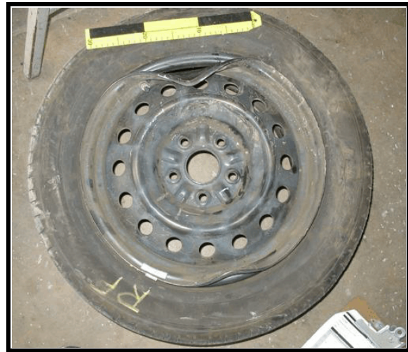
Figure 5. Right front tire/rim damage
