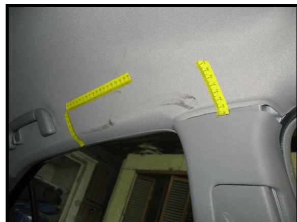
Figure 9. Occupant contact along left roof side rail
