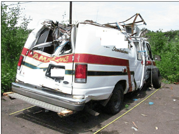
Figure 6: The top of the patient compartment was destroyed and the patient loading doors were damaged during the rollover
