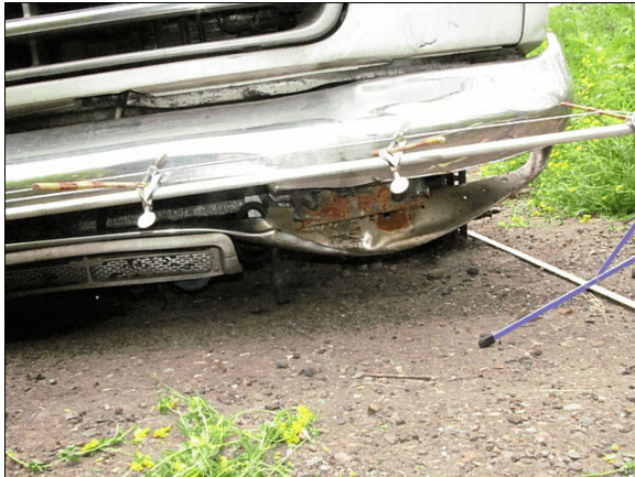
Figure 4: Damage on the front bumper of the ambulance from the impact with the guardrail
