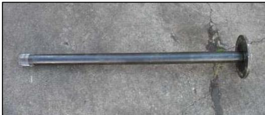
**Figure 8. Removed right drive axle.**
