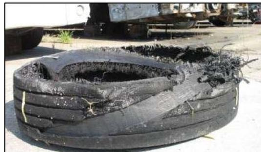
**Figure 11. Partial post-incident tread separation with fire damage across the tire tread.**
