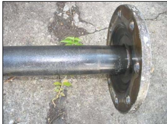
**Figure 9. Close-up view of the outboard end of the axle and the axle flange.**
