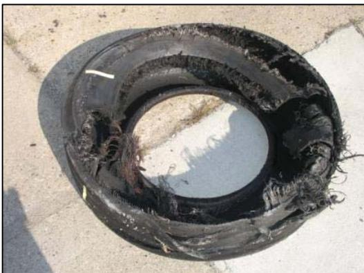
**Figure 10. Inboard sidewall damage to the right inner drive axle tire.**
