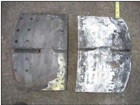
**Figure 12. Heat damage/erosion of the right drive axle brake shoe linings.**
