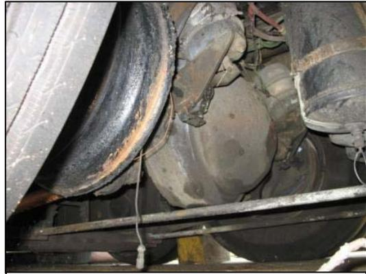
**Figure 5. Fire area the involved the right driver axle undercarriage.**
