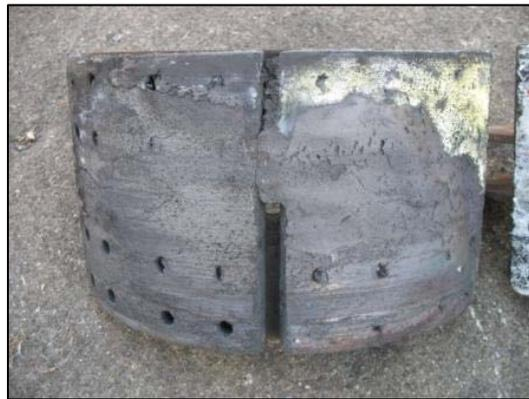
**Figure 13. Close-up view of the damage to the brake shoe lining.**
