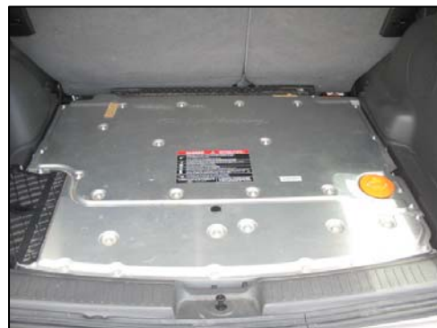
Figure 8: Hybrid battery centered over rear axle and behind rear seat of the Ford Escape.
