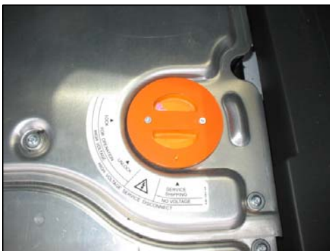
Figure 7: Hybrid battery disconnect switch in the Ford Escape.
