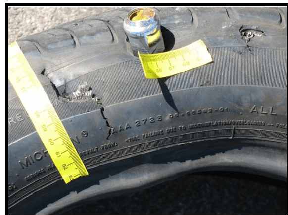
Figure 16. Left front tire damage, 2006 Dodge Charger
