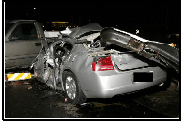
Figure 18. Left and rear damage to Dodge Charger (police photo)
