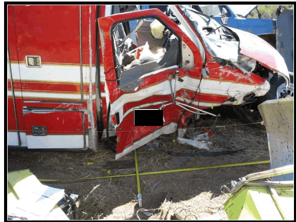
Figure 6. Right side damage (subject vehicle)
