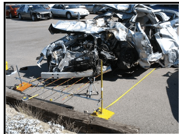
Figure 17. Frontal damage, 2006 Dodge Charger
