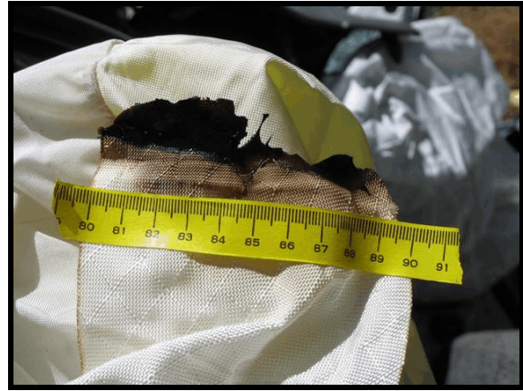
Figure 14. Melted tether strap (subject vehicle)
