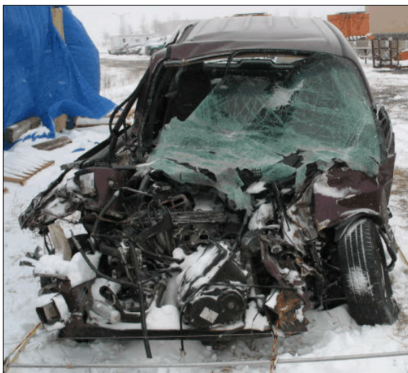
Figure 6: Overview of damage to front of Plymouth from impact with right side of the Thomas bus
