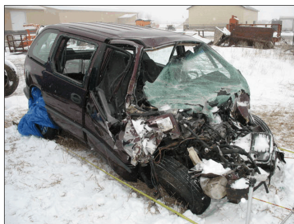
Figure 20: Overview of damage to front of Plymouth from impact with right side of the bus
