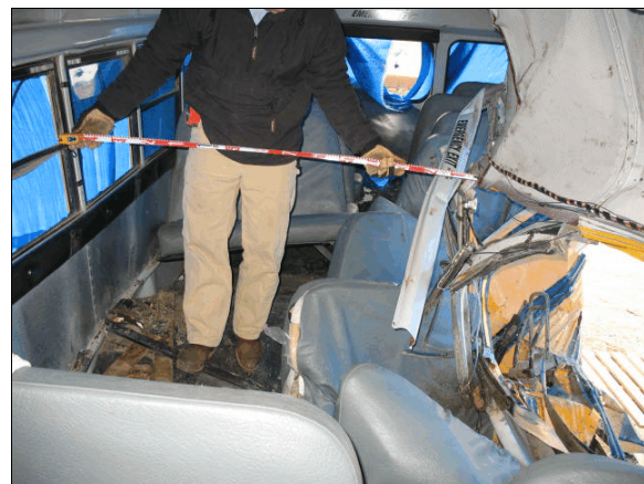
Figure 19: Closer view of left side intrusion involving primarily seat rows 8-11
