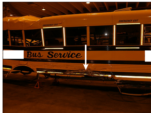
Figure 7: Police photo showing Plymouth's impact location on right side of bus (arrow)
