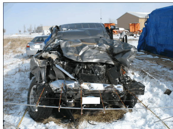
Figure 9: Damage to front of Chevrolet from the impact with the left side of the bus
