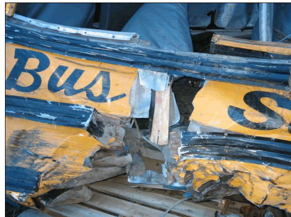
Figure 17: Sheet metal damage to left side of bus
