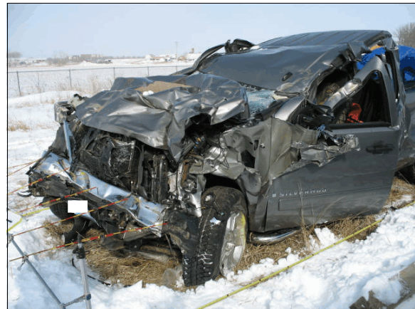
Figure 21: Front left view of damage to the Chevrolet due to the impact with the left side of the bus
