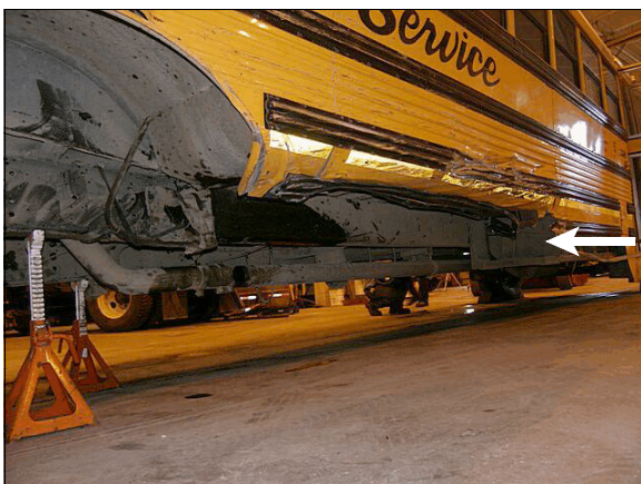
Figure 8: Police photo showing contact to bus' right frame rail; arrow shows location of fuel tank
