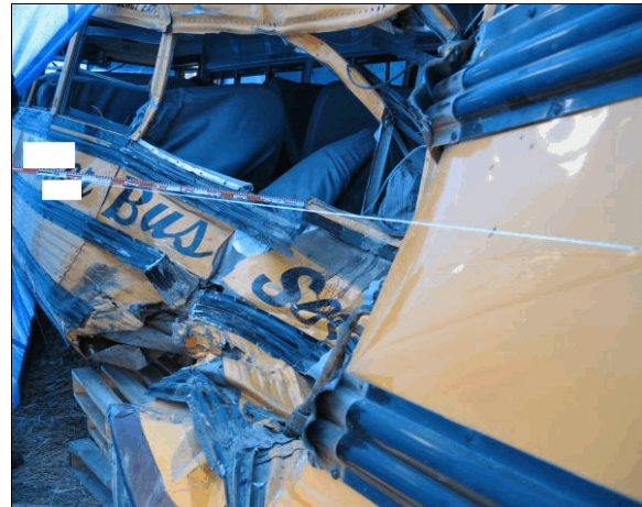
Figure 16: Crush to left side of bus due to impact with Chevrolet; tape measure in tenths of meter
