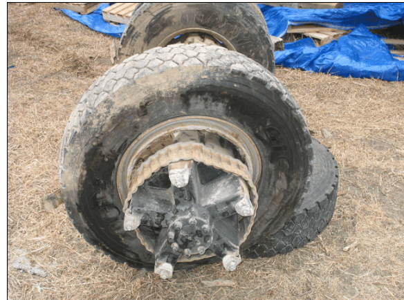
Figure 11: Damage to bus' left rear wheels from impact with the Chevrolet
