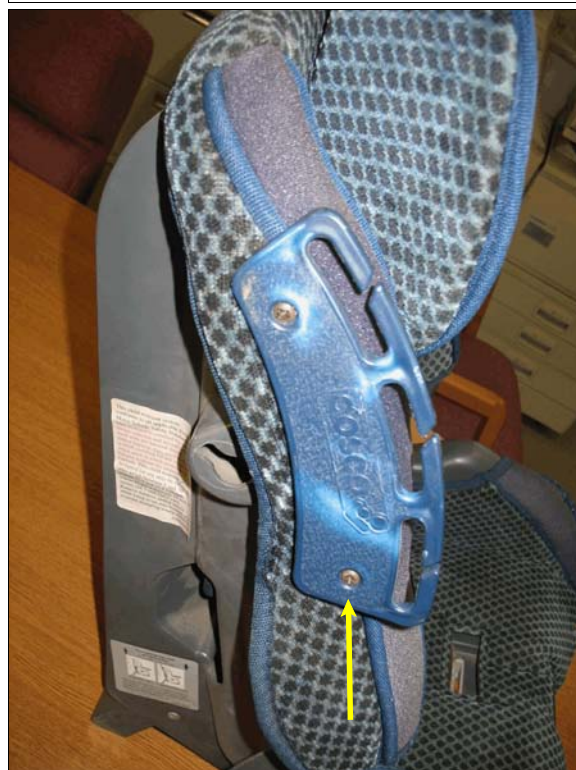
Figure 29: Right (outboard) shoulder belt guide on CSS used by second row right passenger showing white stress marks from loading on guide; Note: screw (arrow) pulled out of seat's plastic frame
