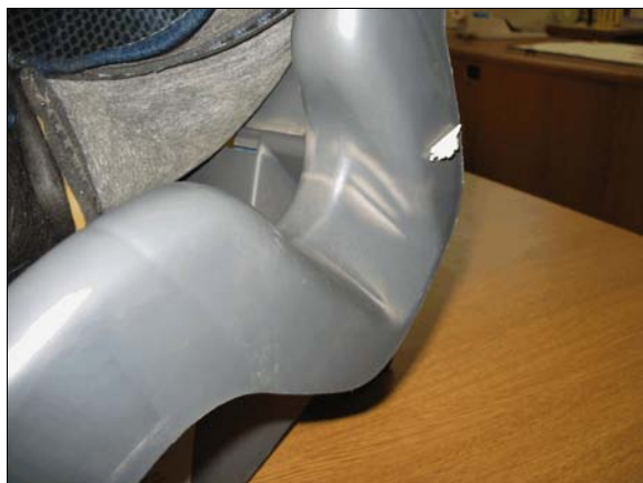
Figure 24: Stress marks on inboard side of Cosco child safety seat's left lap belt guide
