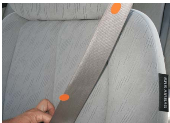
Figure 17: Loading evidence on torso portion of safety belt for Hyundai's driver; Note: tag identifying location of driver's non-deployed, seat back-mounted, side impact air bag
