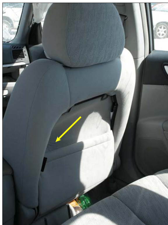
Figure 15: Hyundai's back surface of front right seat back showing contact evidence (arrow) from back right passenger and/or child safety seat
