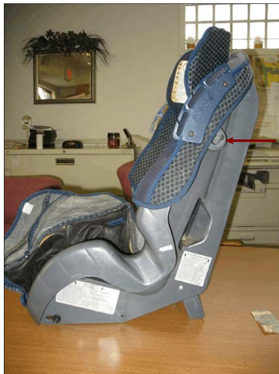
Figure 23: Left (inboard) side of child safety seat used by Hyundai's second row right passenger; arrow denotes location where tray-shield attaches
