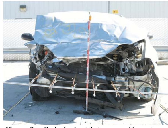
Figure 8: Dodge's frontal damage with contour gauge set at bumper level
