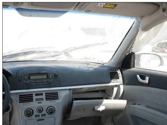
Figure 14: Hyundai's front right seating area showing non-deployed air bag and no evidence of occupant contact; Note: dislodged glove box door
