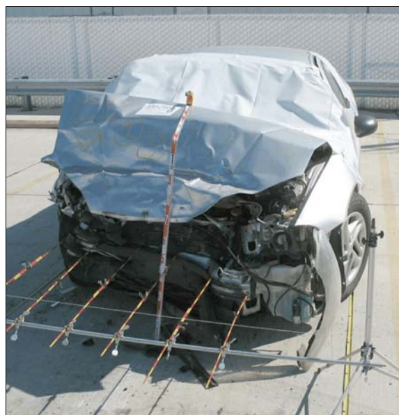
Figure 33: Dodge's frontal damage viewed from left of front; Note: measurement location of C 6 and rightward movement of crush profile
