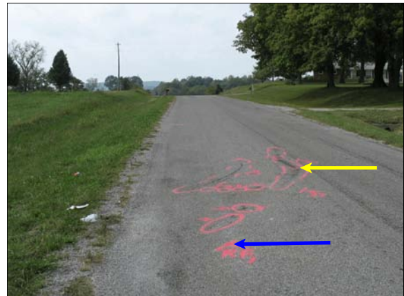
Figure 10: Westerly view showing Dodge's path to impact; Note: back arrow indicates impact scuff and point of deflection for left front tire, and front arrow indicates final rest position of Hyundai's right front tire
