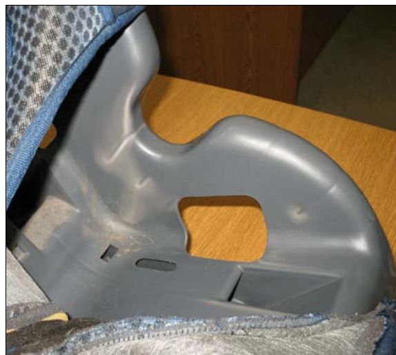
Figure 25: Stress marks on outboard side of Cosco child safety seat's left lap belt guide
