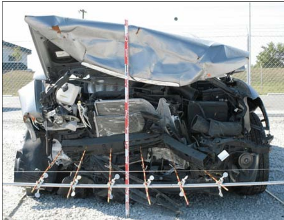
Figure 7: Hyundai's frontal damage with contour gauge set at bumper level
