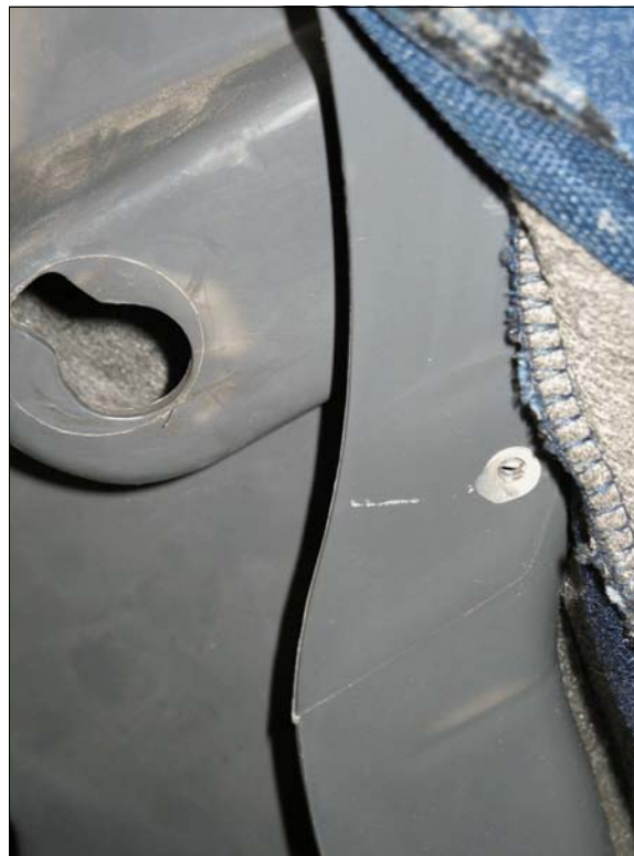
Figure 30: Close-up of location on CSS's plastic frame where screw holding right (outboard) shoulder belt guide pulled out
