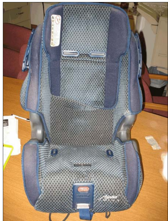
Figure 22: Cosco Alpha Omega, convertible child safety seat used in forward-facing position by Hyundai's second row right passenger as a high-back, belt-positioning booster seat
