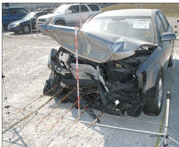
Figure 11: Hyundai's frontal damage viewed from left of front; Note: measurement location of C 6 and rightward movement of crush profile
