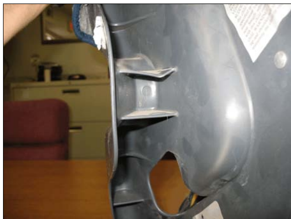
Figure 26: Close-up of stress damage behind left lap belt guide of CSS used by Hyundai's second row right passenger
