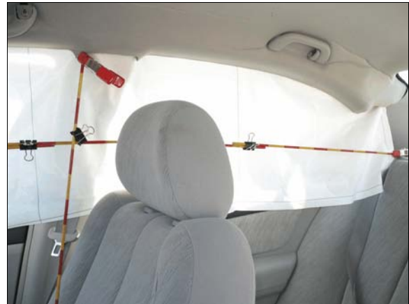
Figure 21: Back portion of Hyundai's deployed right side curtain air bag showing no contact evidence on air bag's interior surface
