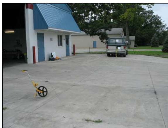
Figure 7: Measuring wheel shows location where target came into surrogate driver's view when looking over right shoulder through backlight
