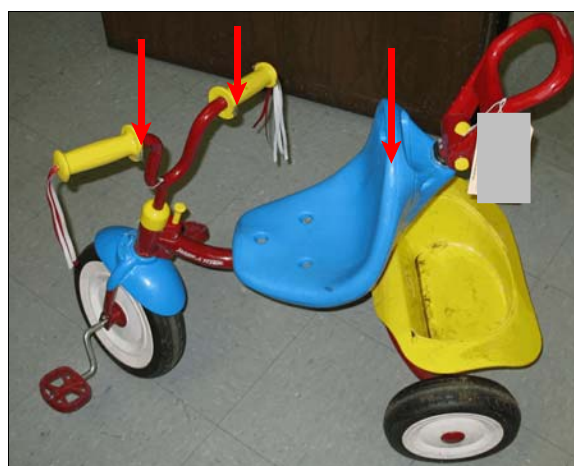
Figure 2: Left side of tricycle, arrows show pavement abrasions
