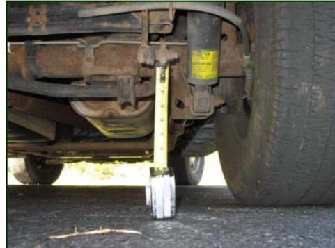
**Figure 6.** Undercarriage components and height of sway bar stabilizer mount.
