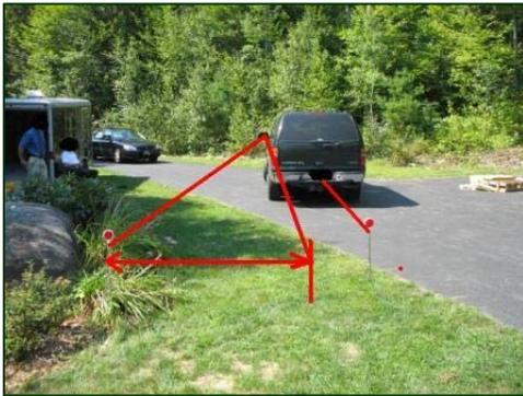
**Figure 13. Cone of visibility from left outside mirror.**
