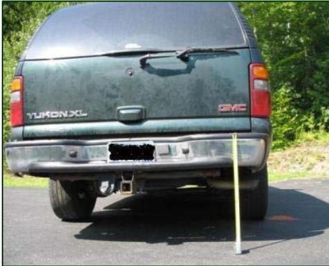
**Figure 5.** Back view and bumper height of the GMC Yukon.
