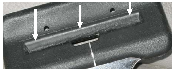
Figure 11: Arrows shows safety belt webbing load abrasions on Isuzu driver's latch plate
