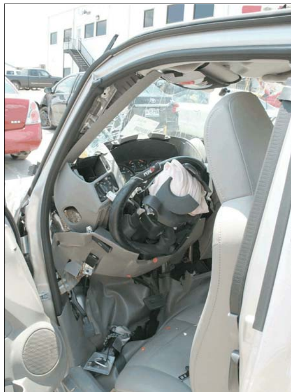
Figure 10: Intrusion of Isuzu's left toe pan and instrument panel and deformation of steering assembly
