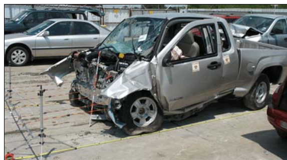
Figure 5: Front left view of damage to front of Isuzu due to impact with the concrete bridge rail; each stripe on the rods is 5cm (2in)
