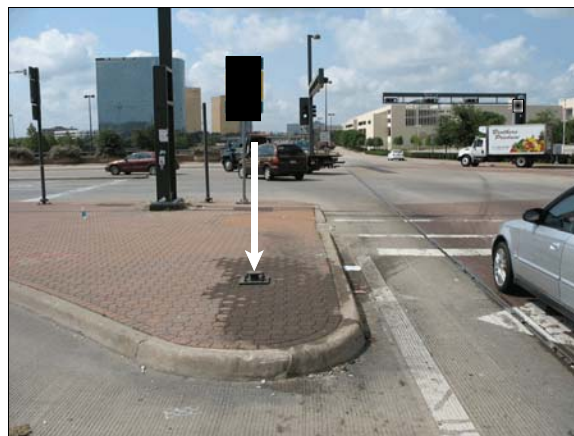
Figure 2: Isuzu's left front and rear wheels impact curb of first traffic island followed by front left impact with sign, arrow shows base of impacted sign.
