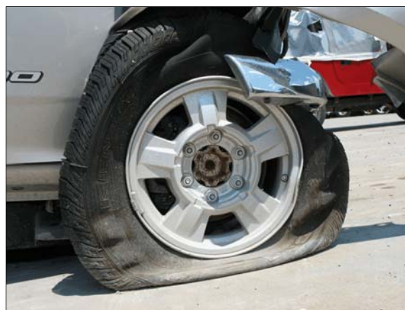
Figure 7: Right front wheel damage from curb impacts.
