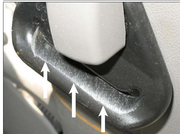
Figure 12: Arrows show safety belt webbing abrasions on Isuzu driver's "D"-ring
