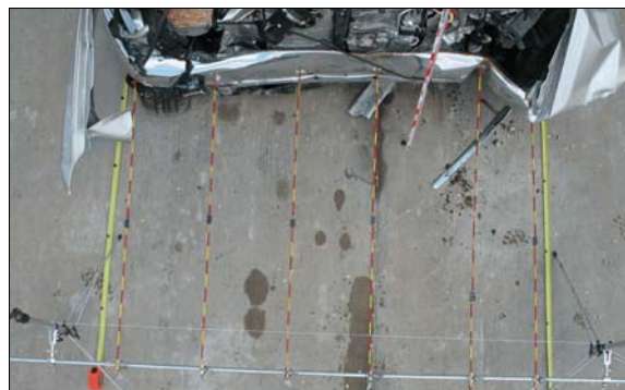
Figure 9: Top view of crush to front of Isuzu due to impact with the concrete bridge rail
