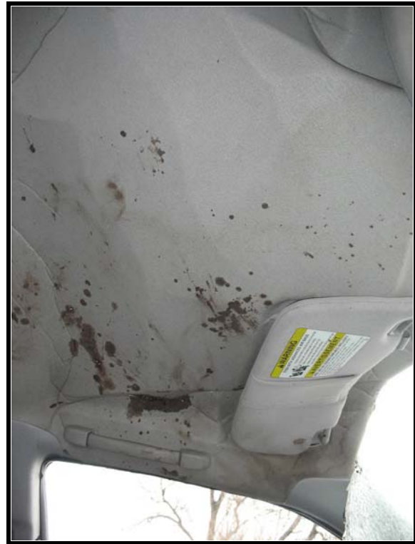
Figure 8. Blood stain pattern and left A pillar movement
