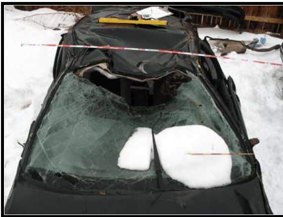
Figure 6. Overview of roof crush
