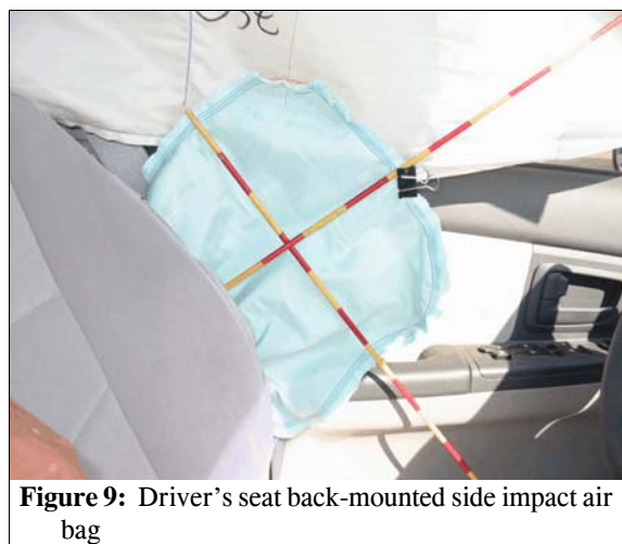
Figure 8: Driver's seat back-mounted side impact air bag located in outboard side of driver's seat back
