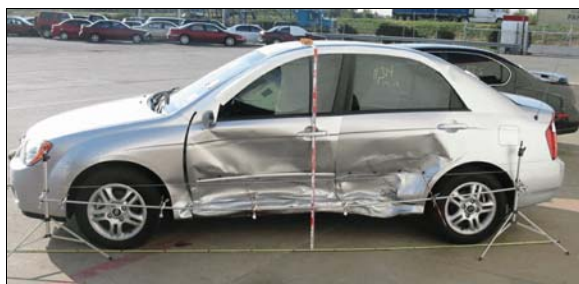
Figure 3: Damage to left side of case vehicle from impact with Nissan, vertical scale incremented in tenths of meter.
