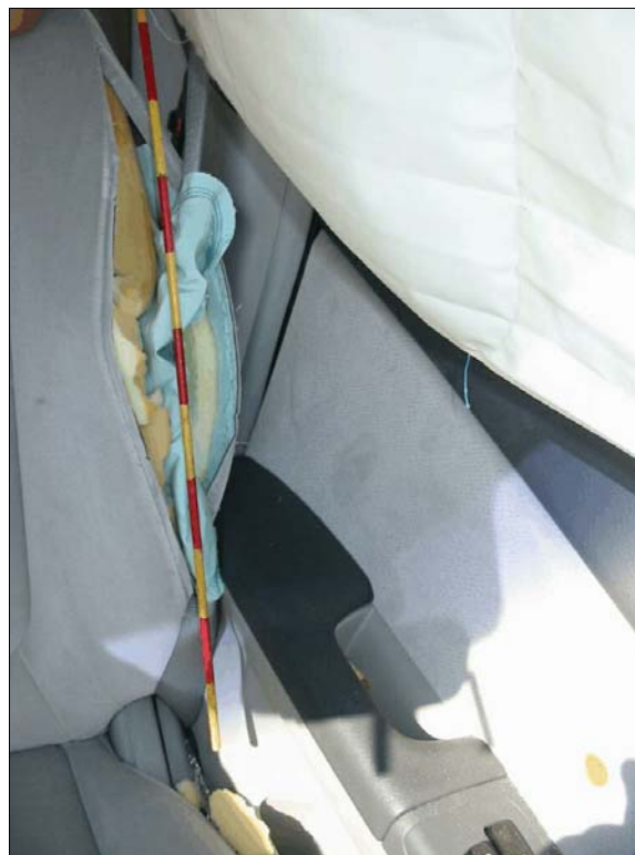
Figure 8: Driver's seat back-mounted side impact air bag located in outboard side of driver's seat back
