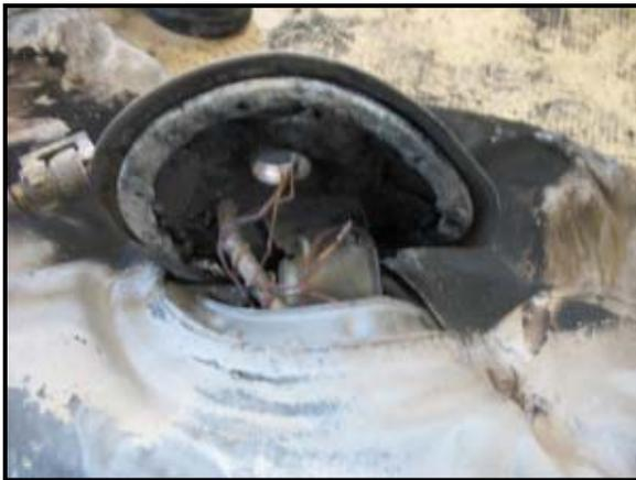
**Figure 18. Displaced sending unit from forward aspect of tank.**
