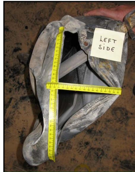
**Figure 19. Ruptured left side of the fuel tank with filler tube in place.**
