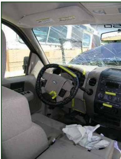
Figure 15. Driver's trajectory and contact points.
