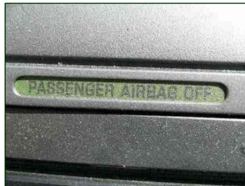
Figure 12. Passenger air bag on/off status lamp.
