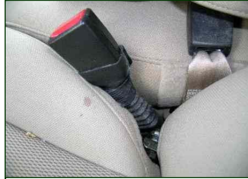
Figure 10. Non-fired driver's buckle pretensioner.
