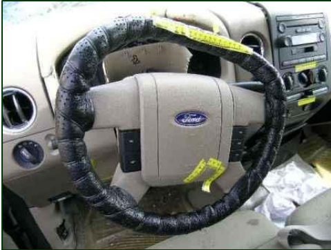
Figure 7. Deformation to the steering wheel rim.
