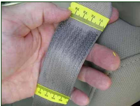
Figure 13. Belt guide abrasion on the shoulder belt webbing.
