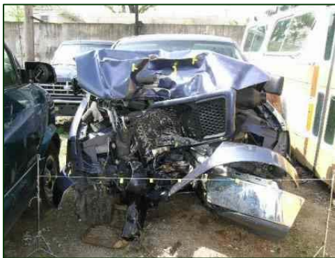
Figure 5. Tree impact damage to the Ford F-150.
