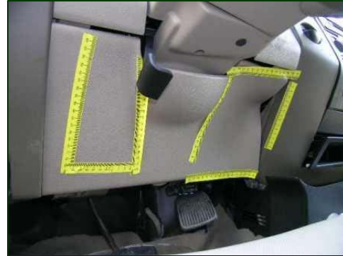
Figure 8. Knee contacts to the rigid bolster panel.
