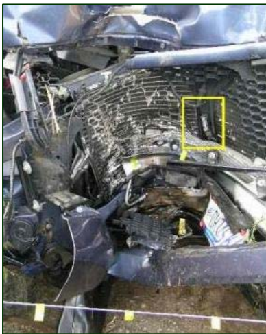
Figure 11. Center front external crash sensor.
