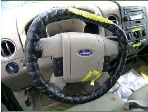
Figure 9. Non-deployed driver's air bag module.
