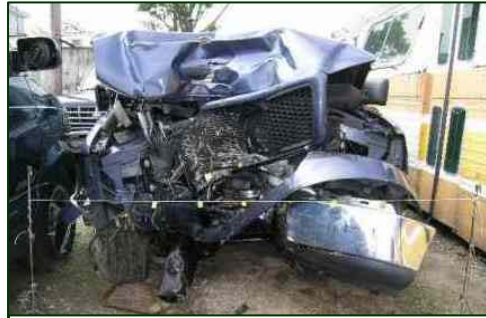
Figure 1. Severe frontal damage to the Ford F-150 pickup truck.
