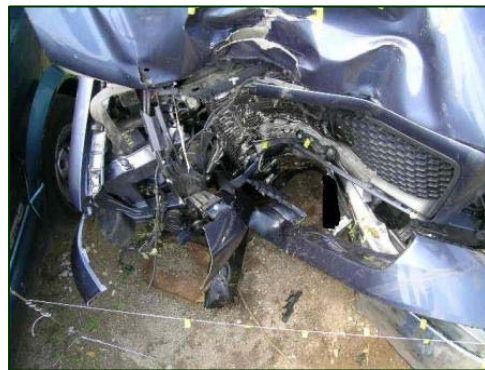
Figure 6. Overhead view documenting the depth of frontal crush at bumper level.
