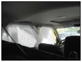
Figure 16: Deployed left side protection.
