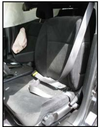
cm to 83 cm (30.0 in to 32.5 in) from the outboard anchor. Examination of the latch plate revealed indicators of historical use. Additionally, the friction surface of the latch plate belt path was abraded indicative of loading. The D-ring was adjusted to the full up position. The surface of the D-ring did not reveal loading evidence. The evidence identified during the examination of the driver's restraint indicated the restraint was in use at the time of the crash.
