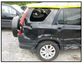
Figure 11: Right rear quarterpanel damage.
