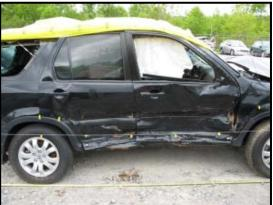
Figure 7: Right side impact damage.
