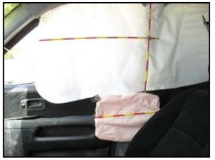
Figure 16: Deployed right side impact protection.
