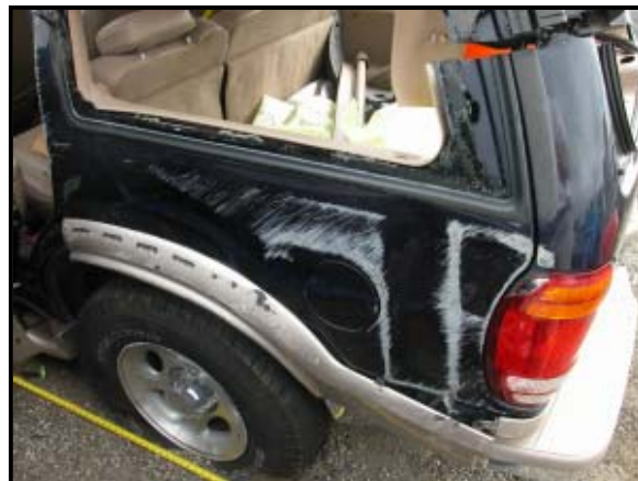
Figure 6: 8/2 o'clock surface abrasions to the left rear quarterpanel of the Ford.
