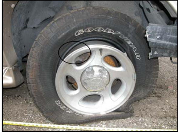
Figure 7: View of the front right tire and rim abrasion.
