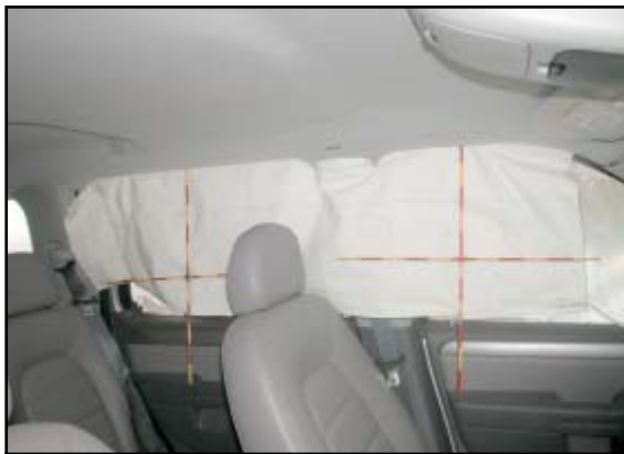
Figure 9. Left side canopy air bag.
