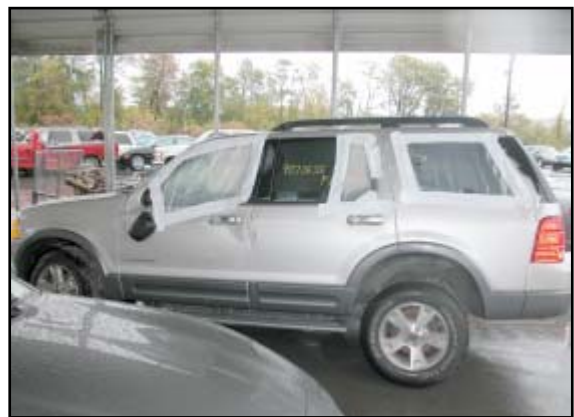
Figure 8. Left side rollover damage.
