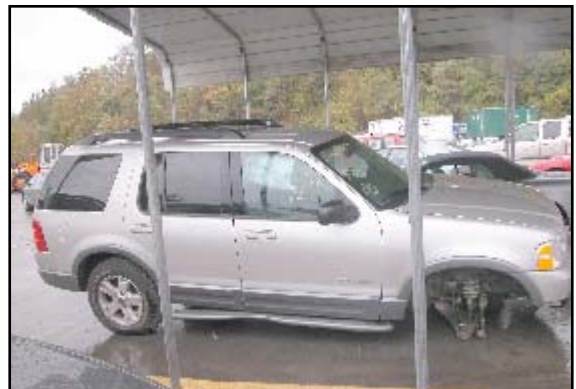
Figure 5. Right step rail damage.
