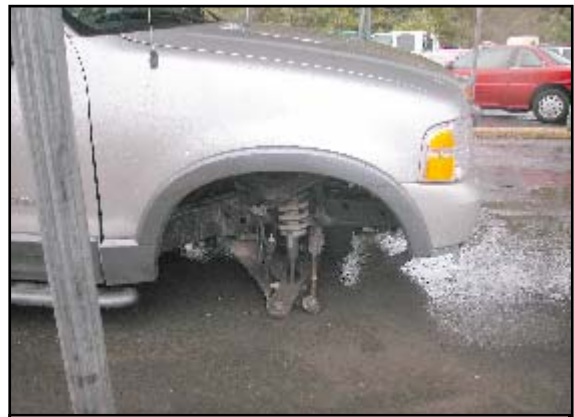
Figure 7. Right front axle damage.
