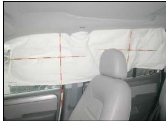
Figure 10. Right side canopy air bag.
