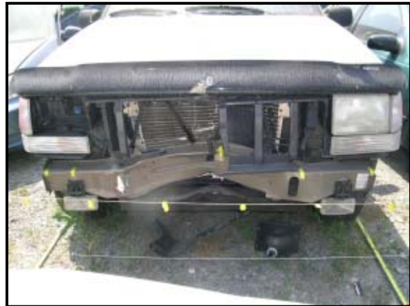
Figure 6: Close-up view of the frontal damage.
