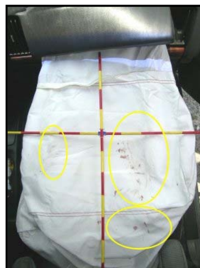
Figure 10: Top surface of the deflated front right passenger air bag.
