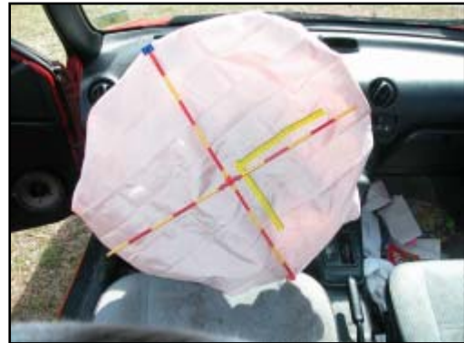
Figure 11. Deployed driver's air bag
