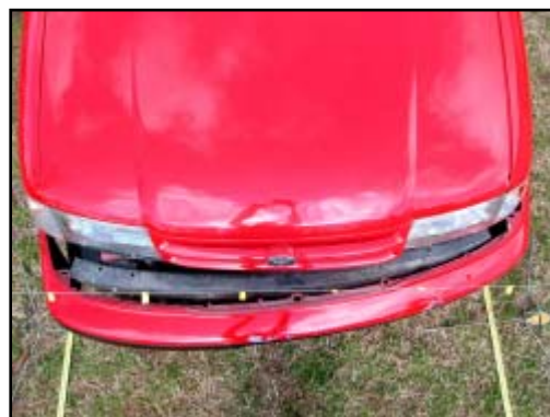
Figure 6. Overhead view of frontal crush profile
