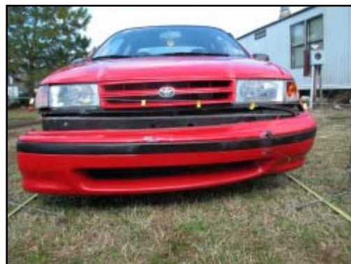
Figure 5. View of frontal damage to bumper fascia
