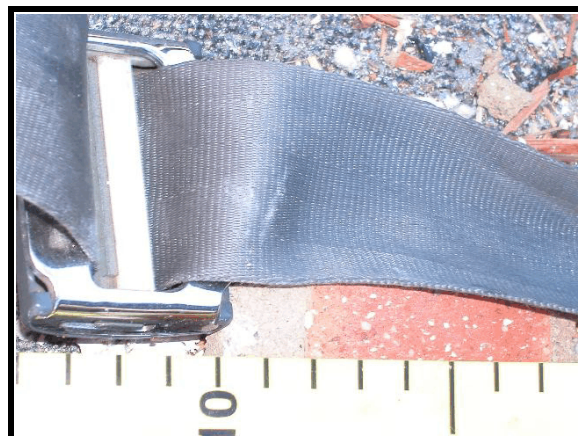
Figure 10. Load marks to middle seat lap belt
