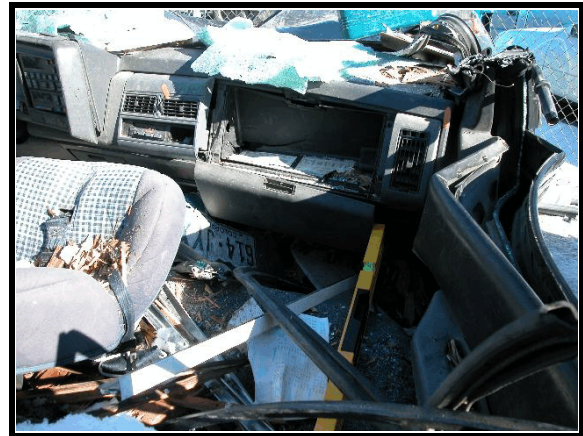
Figure 7. Right door intrusion
