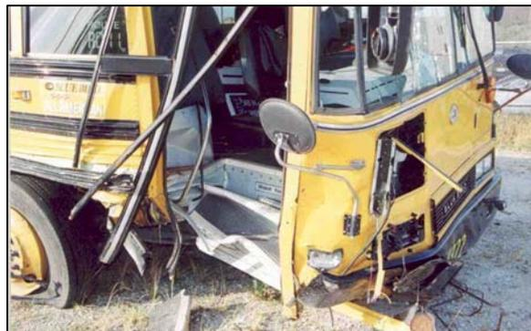
**Figure 4 - Damaged front right corner of bus.**
