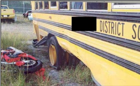
**Figure 5 - Side slap damage to the right side of the bus.**
