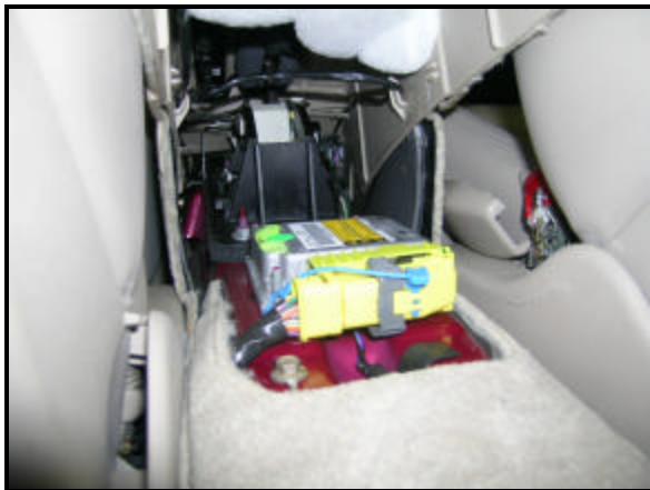
Figure 8: Longitudinal view of the SDM.
