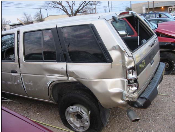
Figure 7: Damage to the left rear corner of Pathfinder from the side-slap impact with the case vehicle, scratches forward of the left rear corner are from the rollover.
