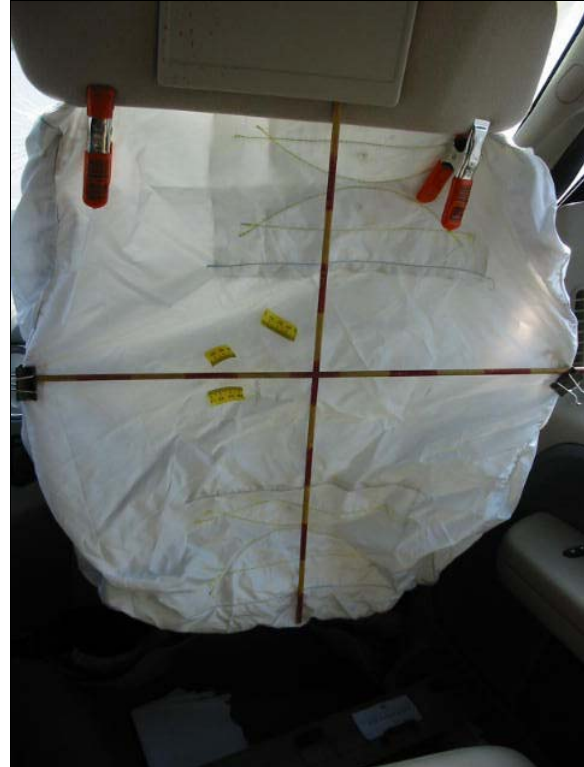
Figure 15: Case vehicle's deployed front right passenger air bag, yellow tape shows area of possible deployment scuffs and possible occupant contact.
