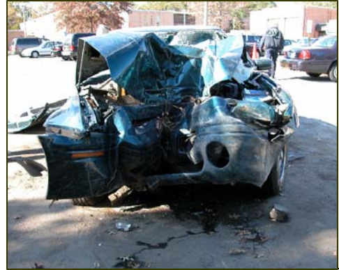
Figure 1. Frontal damage to the 1995 Pontiac Grand Prix.
