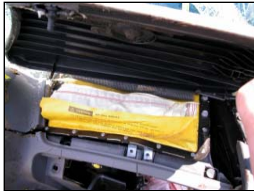
Figure 12. Non-deployed front right frontal air bag.
