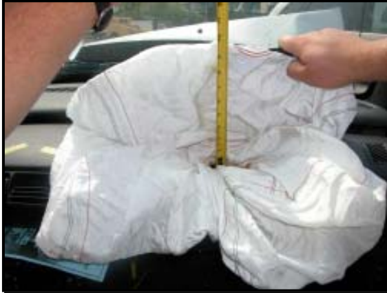
Figure 9: Front right passenger air bag upon initial inspection.
