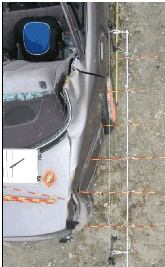
Figure 19: Overhead view of case vehicle's right side damage showing crush profile for BES purposes (case photo #34)
