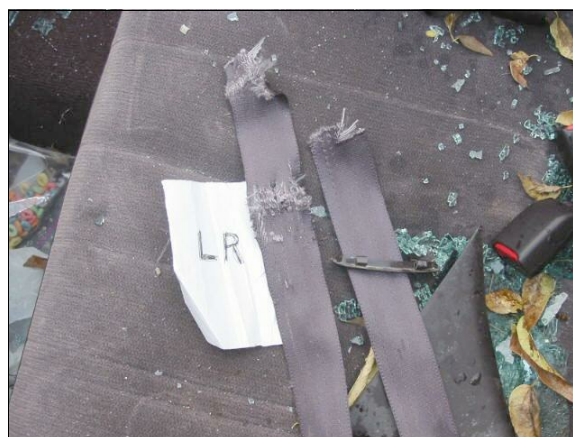
Figure 41: Webbing of case vehicle's back left safety belt showing extrication cuts (case photo #71)
