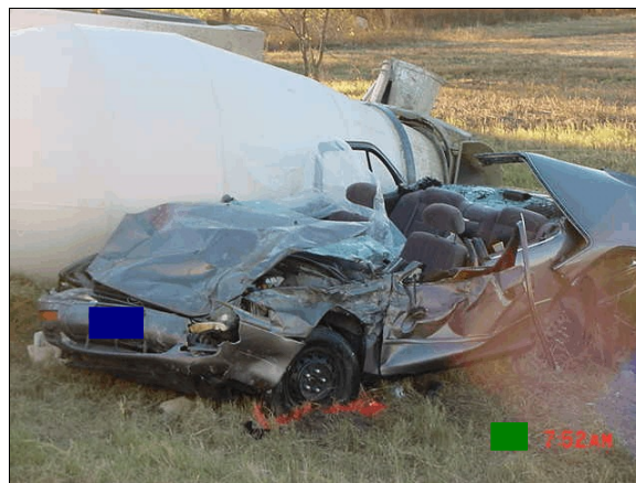
Figure 10: On-scene southeasterly view of final rest positions of Mack truck (background) and case vehicle (foreground); Note: case vehicle's roof and been removed for extrication purposes (case photo #07)
