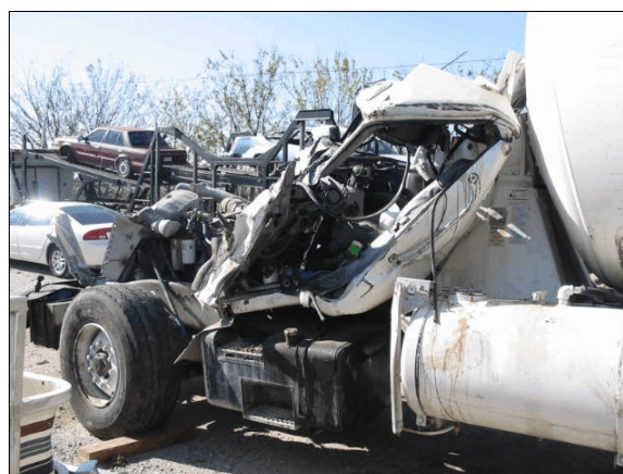
Figure 45: Mack truck's damaged cab area, viewed from back of left; Note: front of case vehicle penetrated into truck's cab while Mack was sliding along on its left side (case photo #113)
