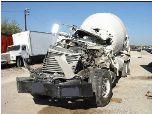
Figure 7: Mack truck's damaged engine and cab areas, viewed from left of front, as a result of case vehicle's penetration impact while Mack was on its left side (case photo #110)
