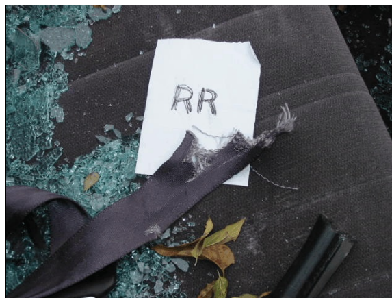
Figure 42: Webbing of case vehicle's back right safety belt showing extrication cuts (case photo #71a)
