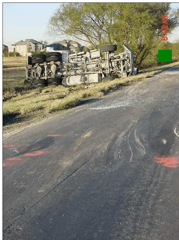
Figure 12: On-scene view of Mack truck's west-southwesterly path on its left side, after rolling over; Note: Mack rotated clockwise as it slid into impact with case vehicle and toward final rest position on south roadside (case photo #15a)
