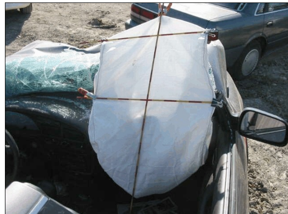
Figure 27: Elevated view of front surface of case vehicle's deployed front right air bag showing no evidence of occupant contact (case photo #65)
