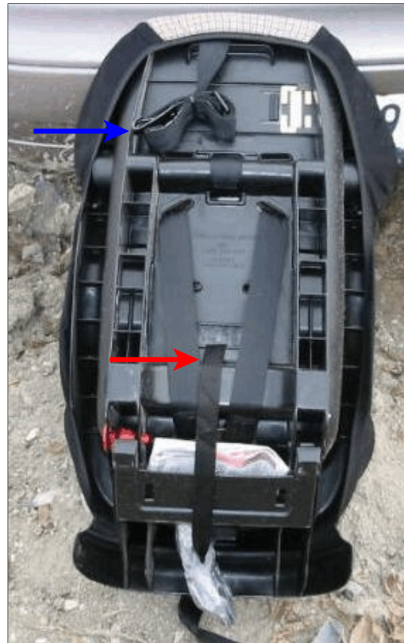
Figure 36: Back surface of case vehicle's Dorel Touriva convertible child safety seat, used in its rear-facing configuration by back right passenger, showing both upper (forward-facing-blue arrow) and lower (rear-facing-red arrow) LATCH attachments and location of instruction booklet (case photo #86)
