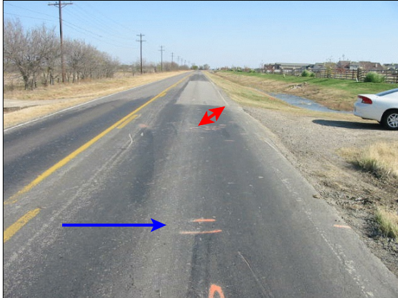
Figure 5: Case vehicle's eastbound travel path at point of impact (blue arrow) with Mack truck which had rolled onto its left side (red arrows) and was sliding in a west-southwesterly direction (case photo #03)
