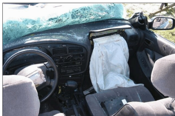
Figure 24: Elevated view of case vehicle's front right seating area showing deployed front right air bag (case photo #45)
