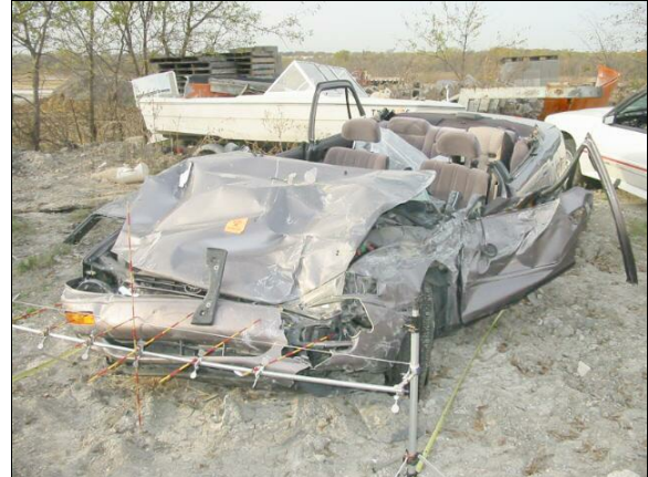
Figure 6: Damage to case vehicle's front, both at and above bumper levels, as a result of vehicle's penetration over Mack truck's engine compartment and into cab area; Note: damage occurred to left side and most likely undercarriage as well (case photo #25)
