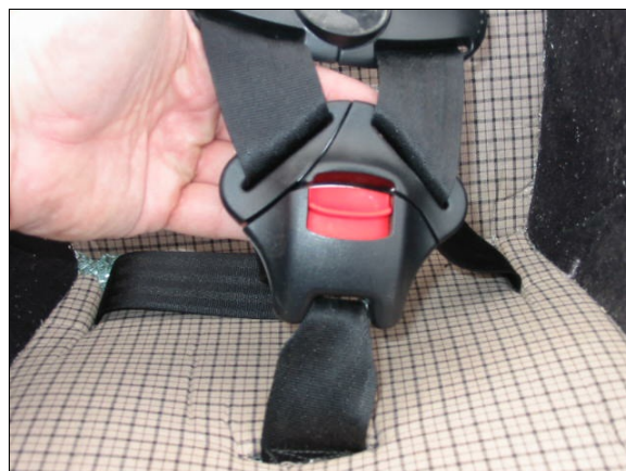
Figure 35: Close-up of five-point, harness system (i.e., fastened) from case vehicle's convertible child safety seat, used in rear-facing configuration by back right passenger (case photo #81)
