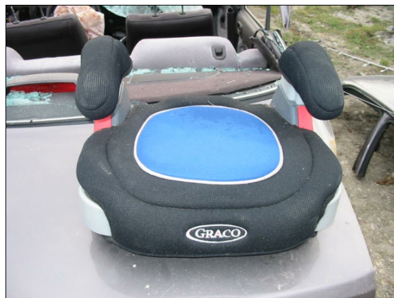
Figure 29: Front of Graco child booster seat used by case vehicle’s back left passenger; Note: seat cushion (i.e., blue on black) folds upward providing “limited” back support for specific children (case photo #99)
