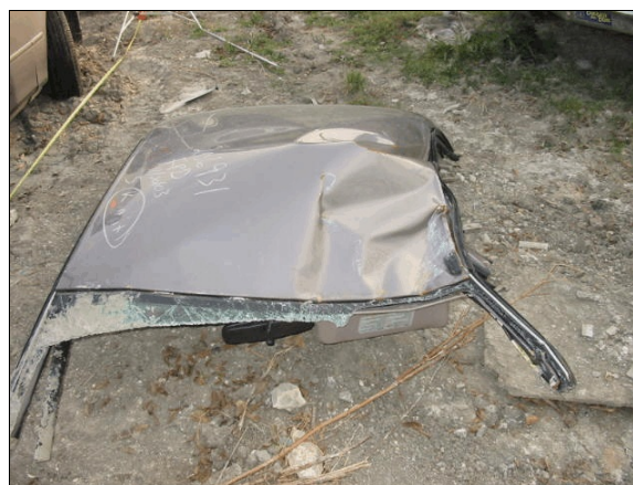
Figure 17: Case vehicle's roof, removed for extrication purposes, showing direct damage above driver's seating area most likely from contact with hood of Mack truck (case photo #23a)
