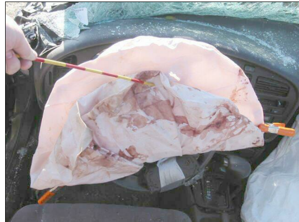
Figure 26: Case vehicle's deployed driver air bag showing copious blood stains on back lower half (case photo #53)
