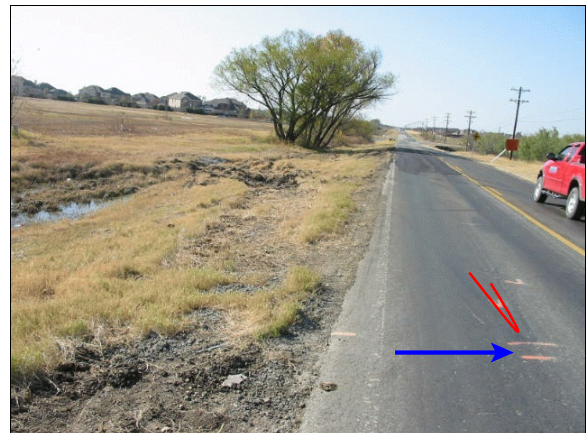
Figure 8: Case vehicle's point of impact (blue arrow) and post-crash travel path; Note: backward deflection path (red line) of rear tire skid mark (case photo #05)
