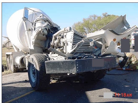
Figure 44: Mack truck's damaged front viewed from right of front; Note: truck was sliding along on its left side when case vehicle struck and overrode engine compartment, penetrating into cab area (case photo #116)
