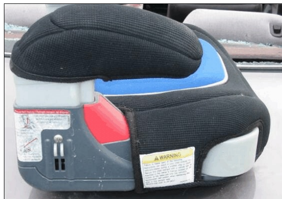
Figure 32: Right side of Graco child booster seat used by case vehicle's back left passenger showing warning label, instructions for securing seat with vehicle's safety belts, and red positioning device for placement of actual seat belt (case photo #102)
