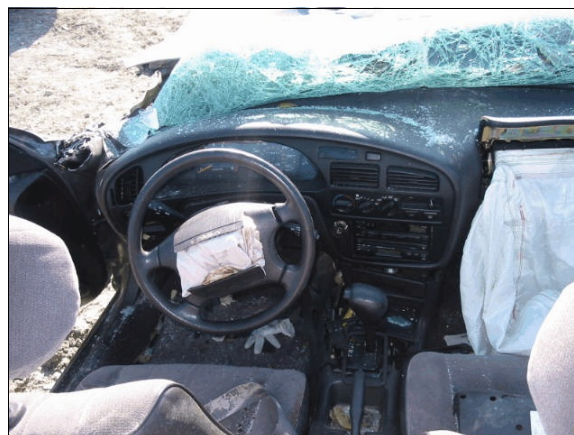
Figure 23: Elevated view of case vehicle's driver seating area showing deployed driver air bag (case photo #43)
