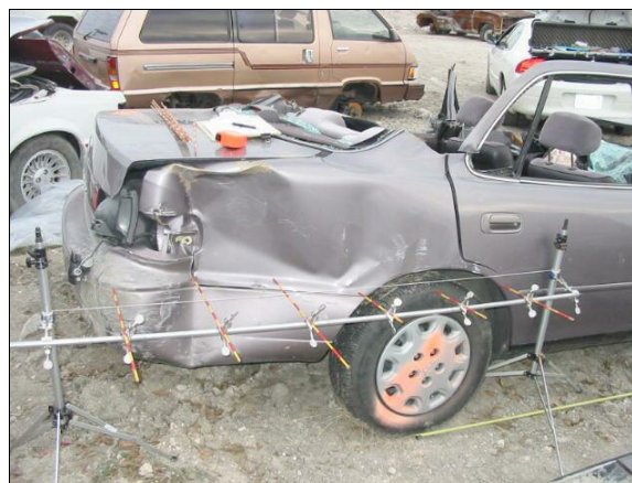
Figure 18: Damage to case vehicle's right quarter panel (3 rd event) from impact by unknown portion of Mack truck's left side during vehicle's counter-clockwise rotation to final rest (case photo #32)
