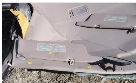
Figure 22: Overhead view of interior surface of case vehicle's roof showing contact evidence on driver's sun visor and roof's windshield header (case photo #62)
