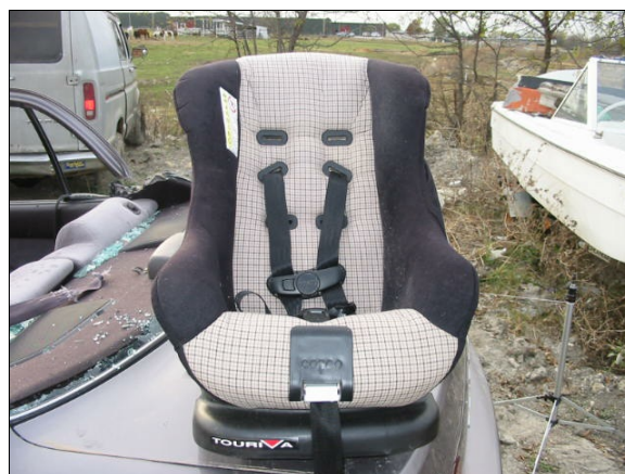
Figure 33: Front of Dorel Touriva convertible child seat used in rear-facing configuration by case vehicle's back right passenger (case photo #80)
