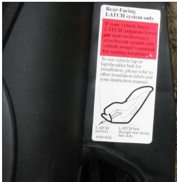
Figure 37: Close-up of manufacturer's label on left side of case vehicle's convertible child safety seat used in rear-facing configuration by back right passenger showing proper method for securing seat's LATCH attachments to vehicle while in rear-facing configuration (case photo #93)
