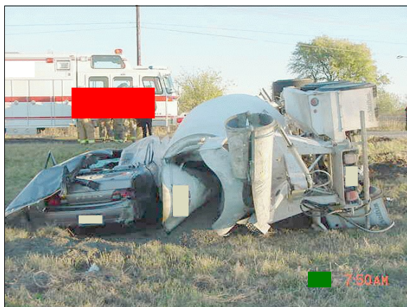
Figure 11: On-scene northern view of final rest positions of case vehicle (left) and Mack truck (right); Note: case vehicle's roof removed for extrication purposes (case photo #08)
