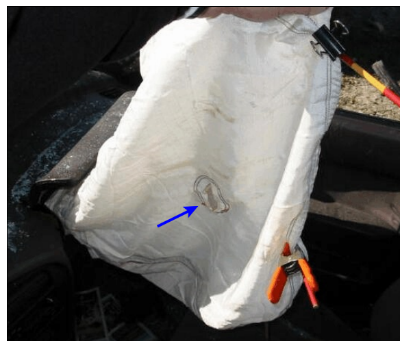
Figure 28: Left side surface—relative to the front right seating position, of case vehicle's deployed front right air bag, showing blood (arrow) on surface near vent port, most likely from driver (case photo #66)
