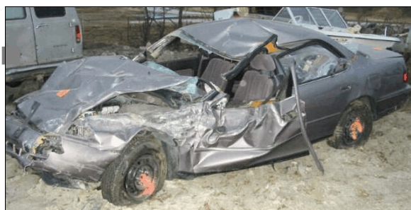
Figure 16: Case vehicle's front and left side damage viewed from front of left with roof, cut for extrication purposes, placed back on top of body (case photo #25a)
