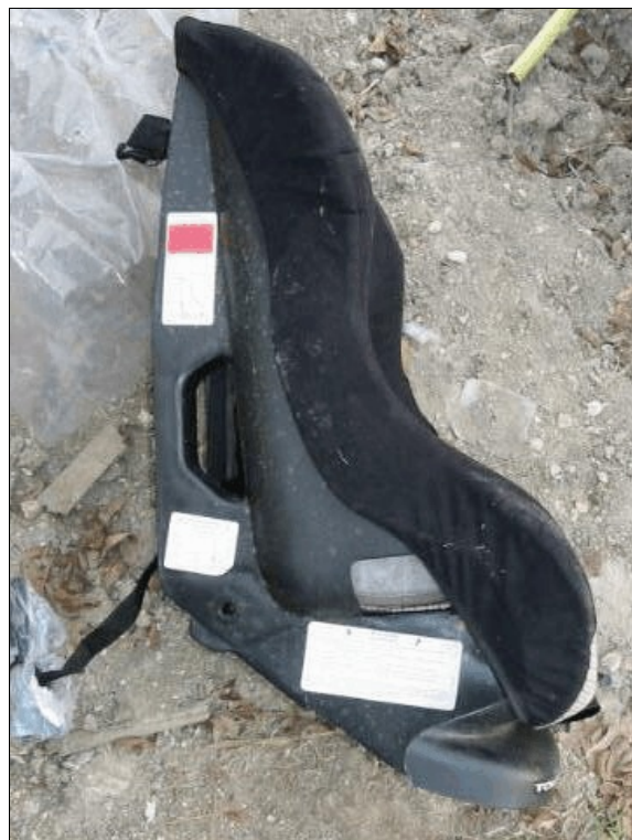
Figure 38: Right side of case vehicle's convertible child safety seat used by back right passenger in rear-facing configuration showing applicable manufacturer's labels (case photo #90)
