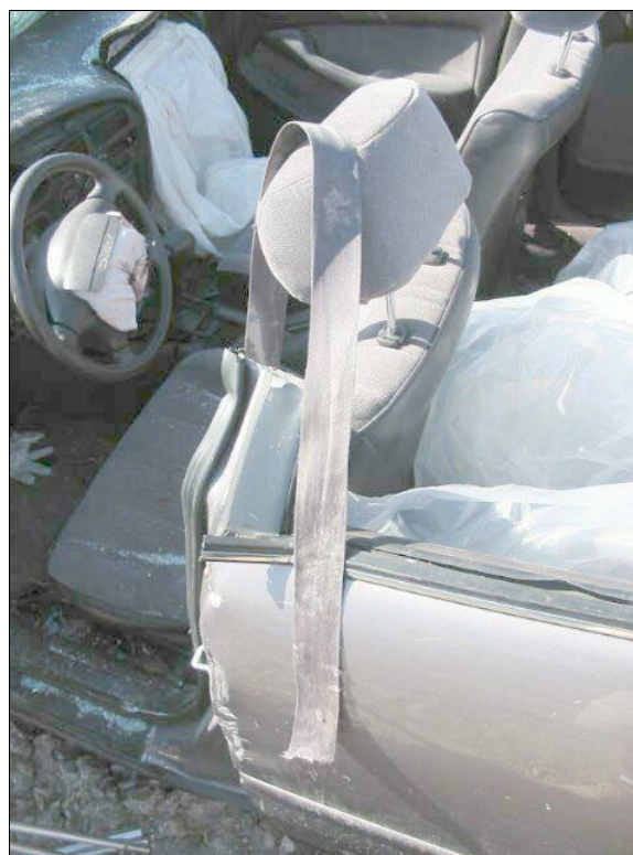
Figure 43: Webbing of case vehicle's driver safety belt showing extrication cuts (case photo #60)
