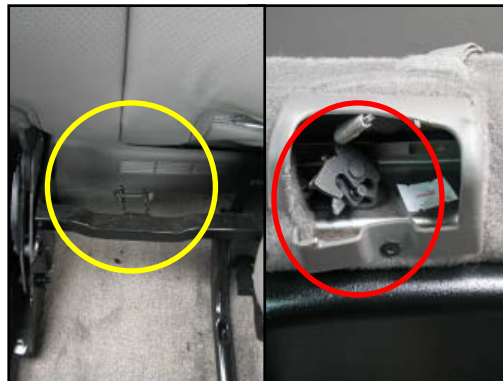
Figure 10. Close-ups of deformed anchor and latch
