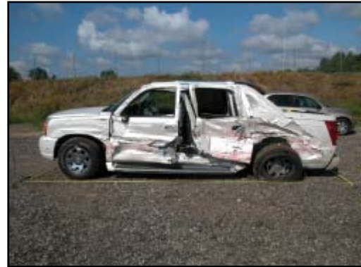
Figure 4. View of left side damage to the Escalade
