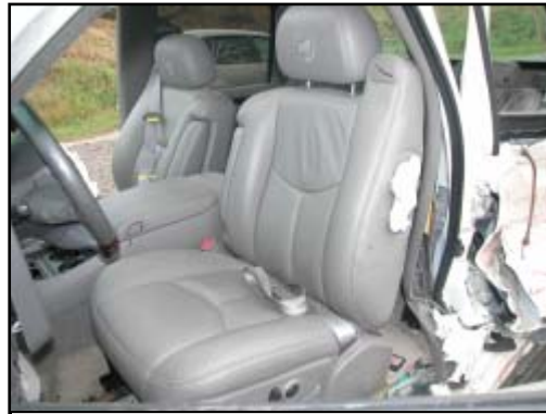
Figure 8. Left side view showing B-pillar intrusion
