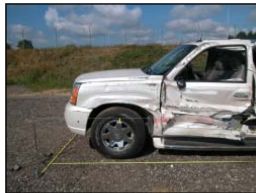
Figure 6. Close-up of abrasions on the front left aspect from the rollover event
