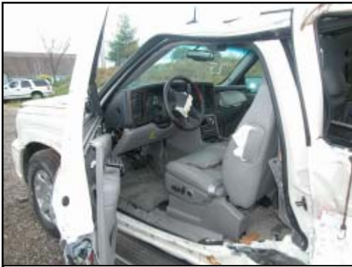
Figure 7. Left side view of intrusions and occupant contacts
