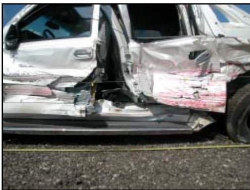
Figure 5. Close-up of separated left B-pillar
